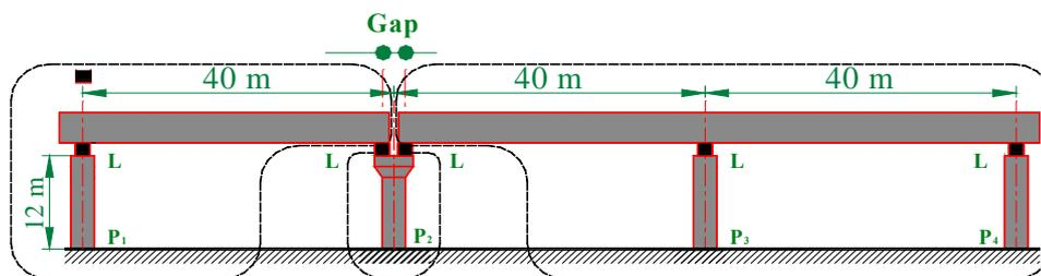
Fig. 1 Base isolated bridge model with LRB bearings (L)
