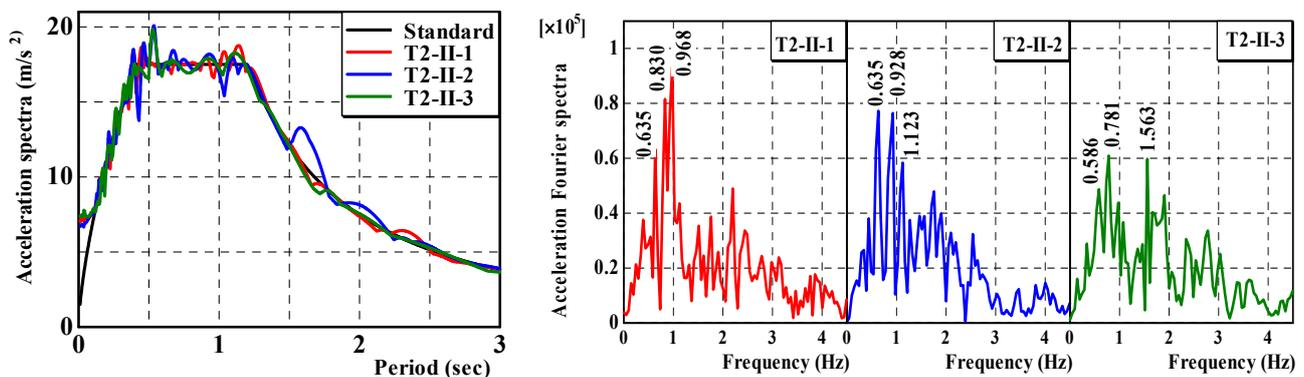
Fig. 4 Acceleration response spectra of the earthquake motions
