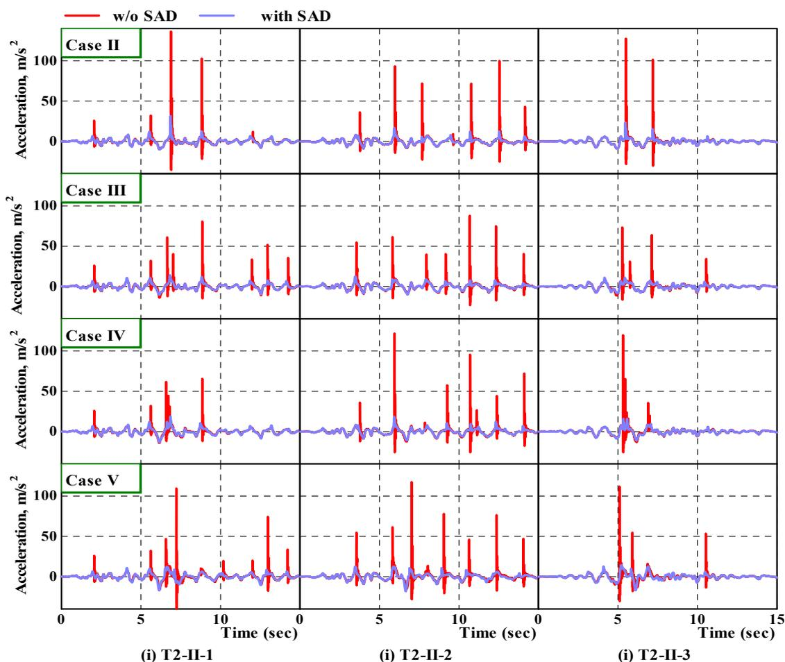
Fig. 9 Deck acceleration time history response with/without SAD
