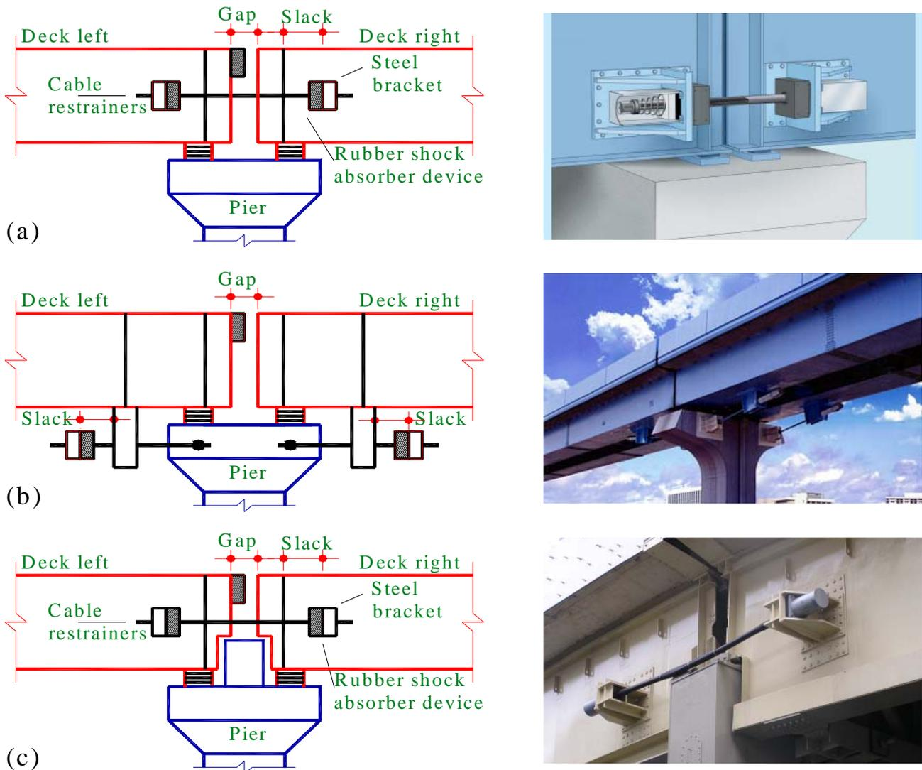
Fig. 2 Schematic of bridge expansion joint with various restrainers configurations: (a) through the hinge – Configuration I, (b) through the pier – Configuration II, (c) through hinge with shear key – Configuration III
