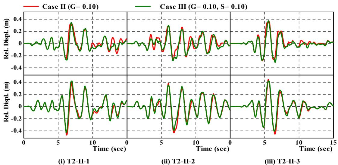
Fig. 7 Relative displacement time history at LRB level
