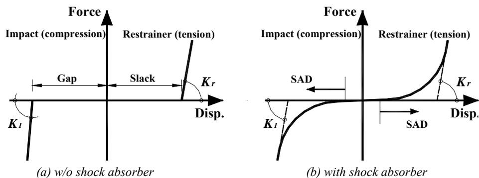
Fig. 3 Pounding, restrainers and shock absorber device (SAD) models
