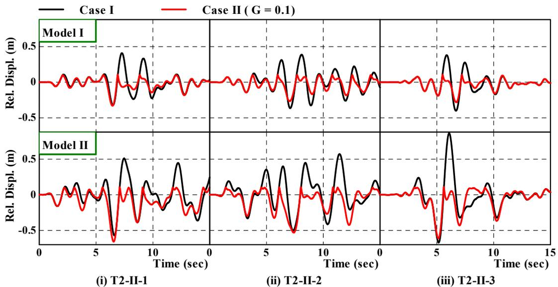
Fig. 6 Expansion joint relative displacement response time history
