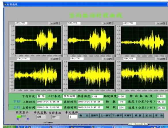
Figure 7 Vertical vibration displacement temporal curves of girder
