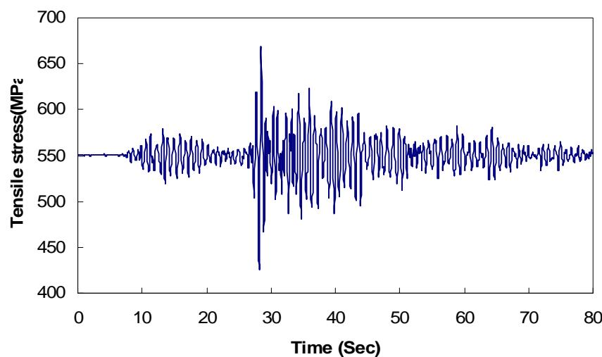
Figure 6 Time History of Tensile Stress in Cable 14
