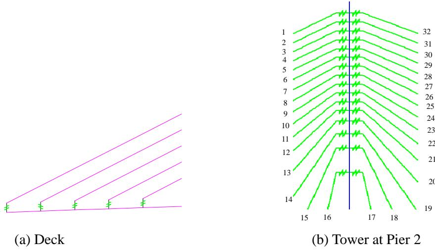
Figure 2 Details of the Deck and Tower Modeling
