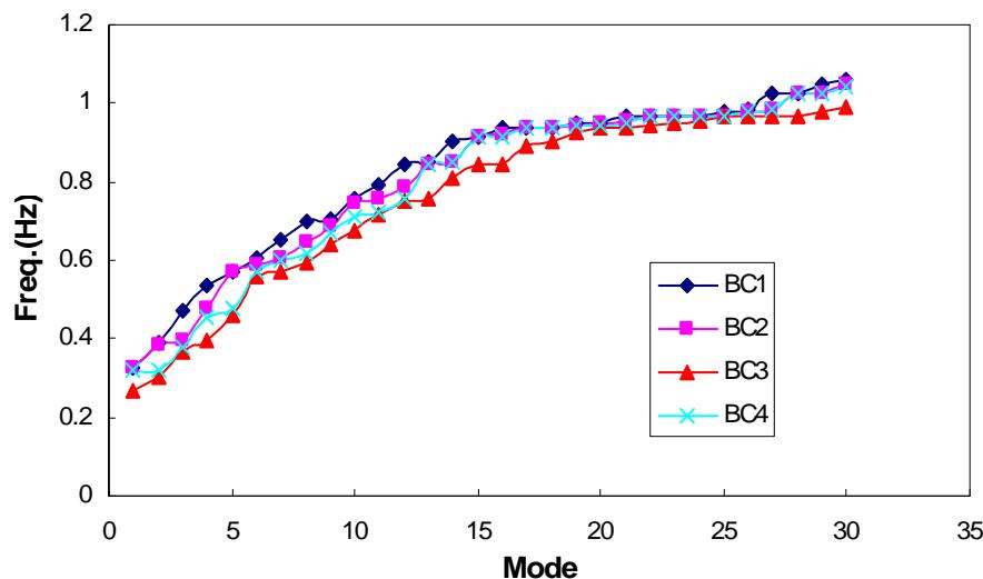
Figure 3 Frequency Variations under Different Boundary Conditions
