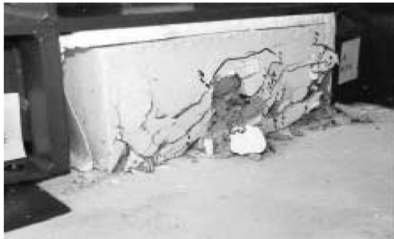
Figure 1- Typical failure mode of concrete shear key [14]
