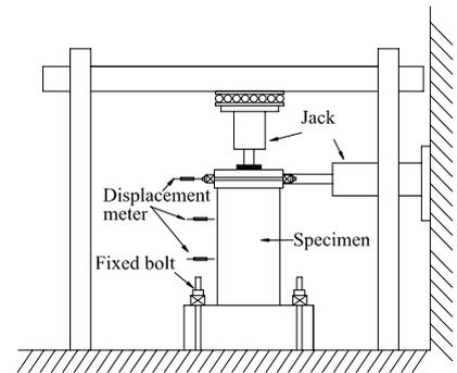
Figure 2 Test set-up
