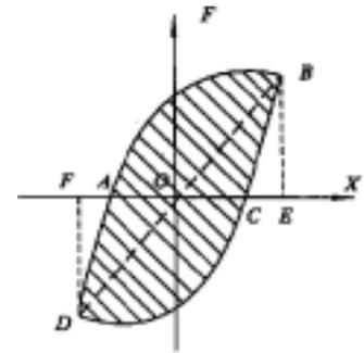
Figure 4 Equivalent viscous damping coefficients of capacity
