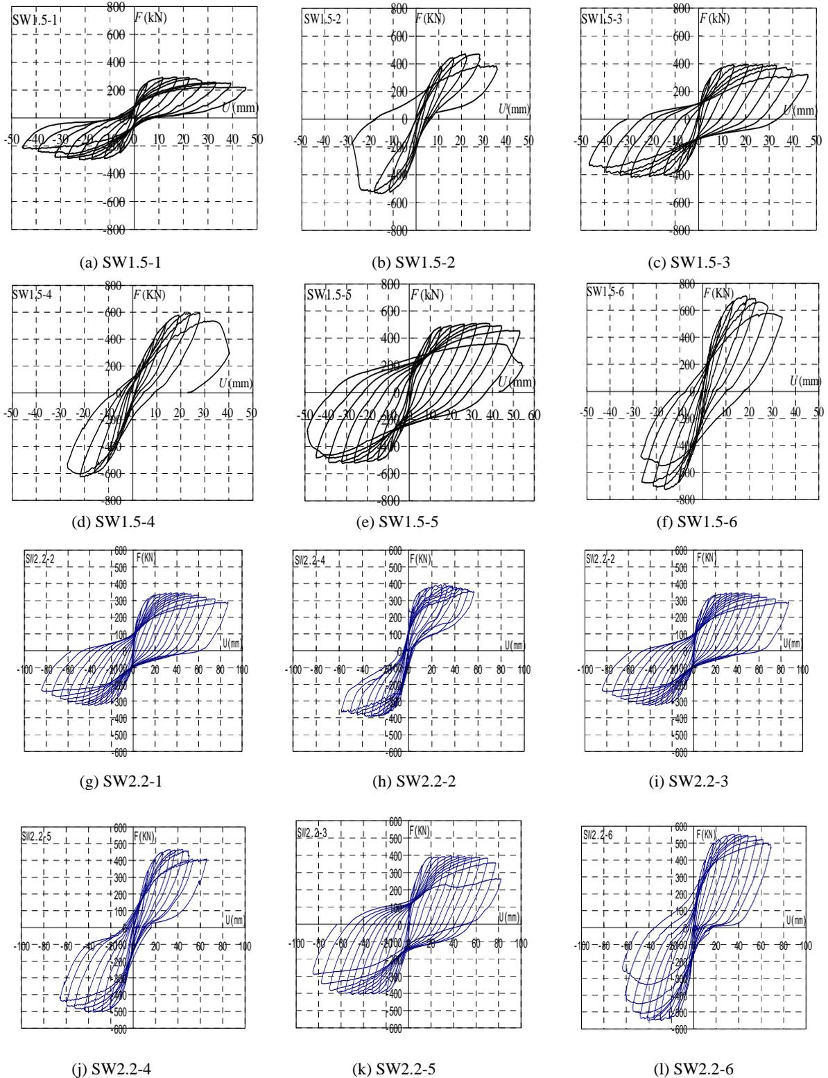
Figure 3 Hysteretic curves of “load-displacement” of specimens
