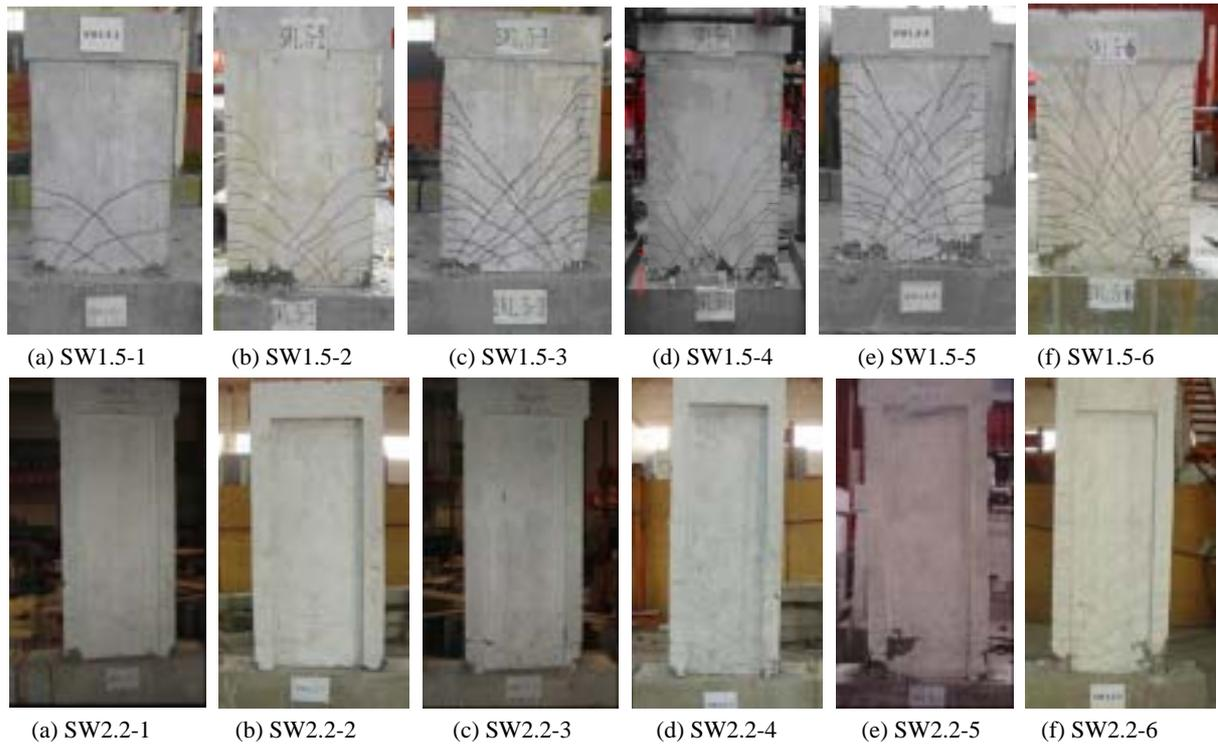
Figure 5 Photos of the specimens at failure
