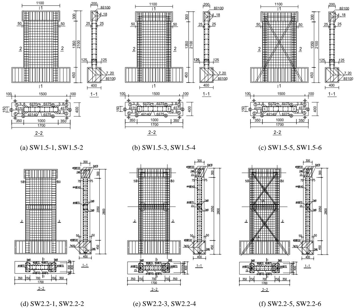
Figure 1 Steel bar and steel details of models
