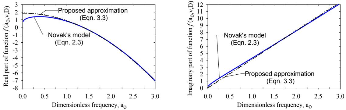
Figure 2 Example of the proposed curve fitting for the real and the imaginary parts of  $f(a_0, \nu, D)$  for  $\nu = 0.5$
