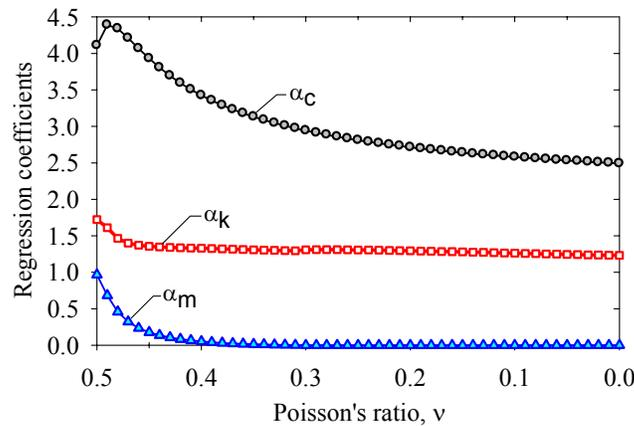
Figure 3 Variation of the regression coefficients with Poisson's ratio from 0.5 to 0.0.
