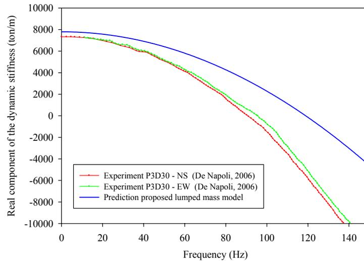
Figure 6 Experimental vs numerical pile dynamic stiffness, real component
