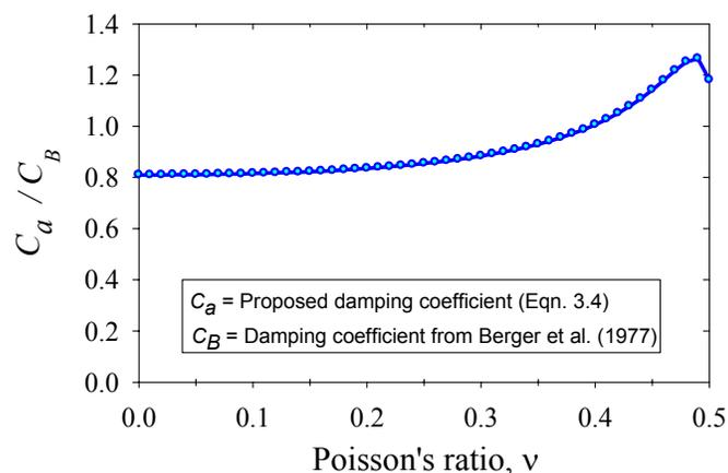
Figure 4 Ratio between damping coefficients  $c_a$  and  $c_B$  for different Poisson's ratios
