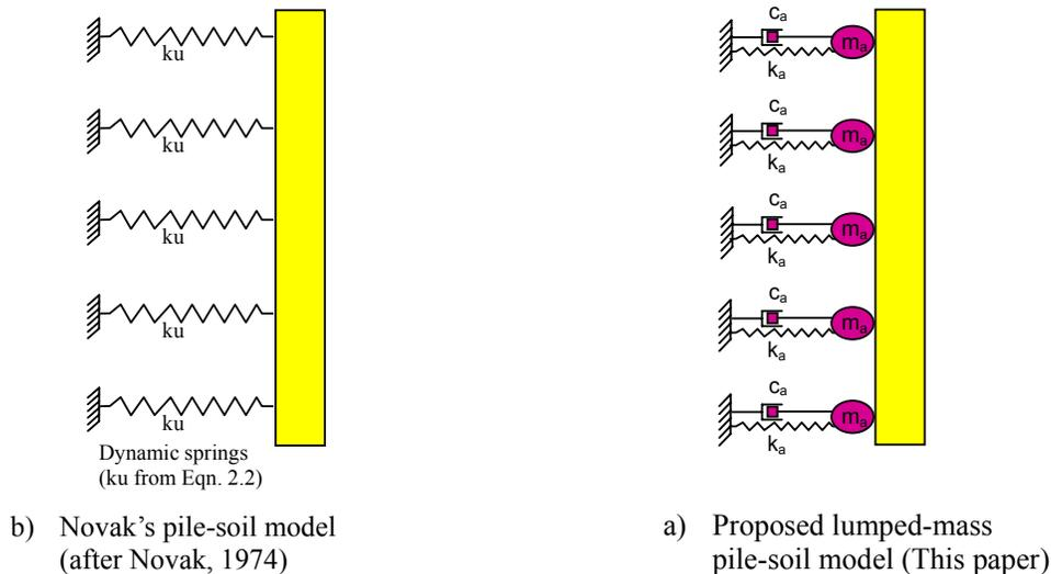
Figure 1 Two dynamic pile-soil models
