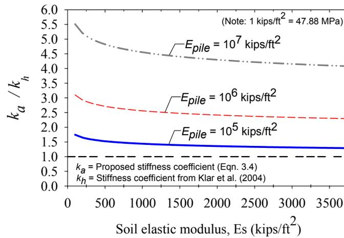
Figure 5 Ratio  $k_a/k_h$  for different moduli of elasticity of the soil and the pile, and Poisson's ratio  $\nu = 0.3$
