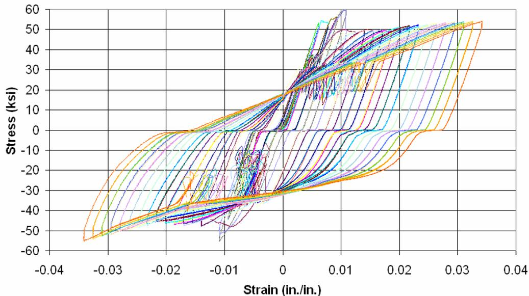
Fig. 4 – BCE Fuse 1-Bar Specimen Typical Hysteretic Behavior (Stress calculated as force divided by cross-sectional area of yield zone. Strain calculated as total deformation divided by the length of the yield zone of the bar).
