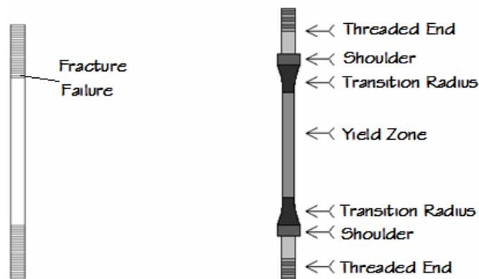
Fig.1 – Preliminary SMA Rod Configuration vs. Carbon Steel Bar Configuration.
