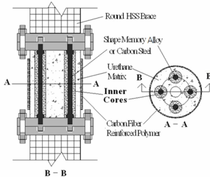
Fig. 2 – BCE Fuse Configuration with Inner Cores.
