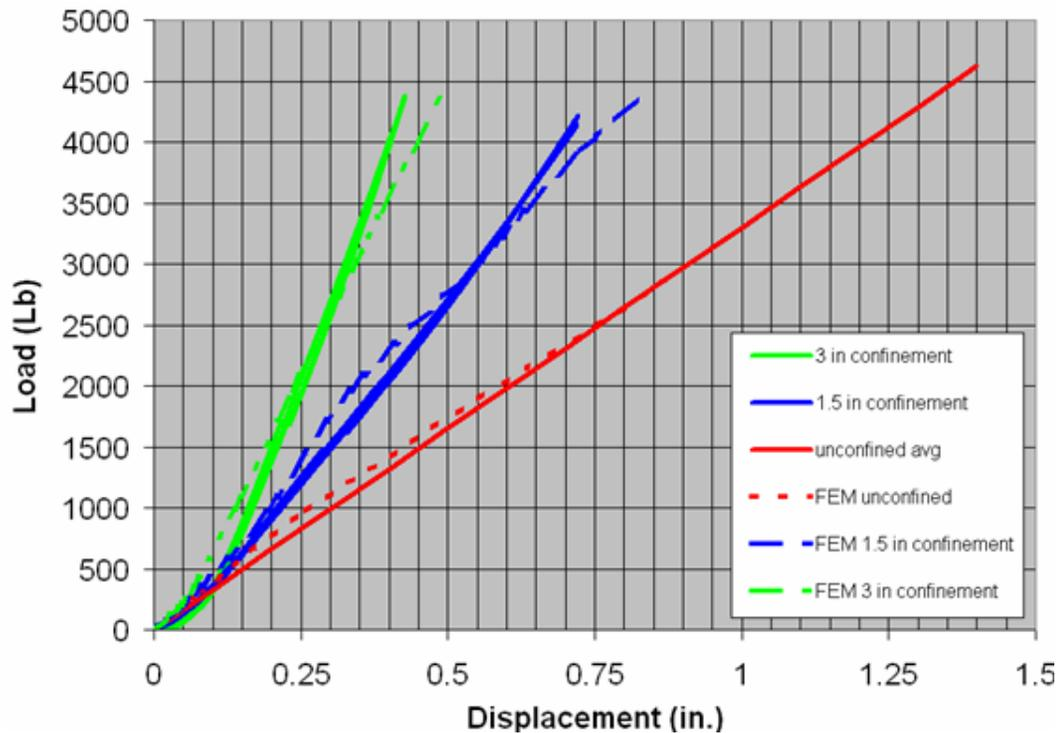
Fig. 3 - Experimental and Computational Load-Deformation Relationships for Urethane-CFRP Assemblies.
