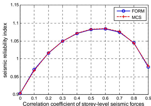
Figure 5 Changing of global seismic reliability index with the correlation coefficient of seismic forces
