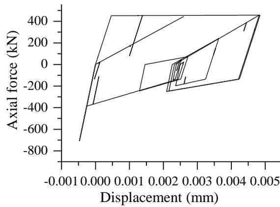
Figure 6. Axial stiffness hysteretic curve of the outside vertical element in the first floor subjected to the peak ground acceleration 220gal
