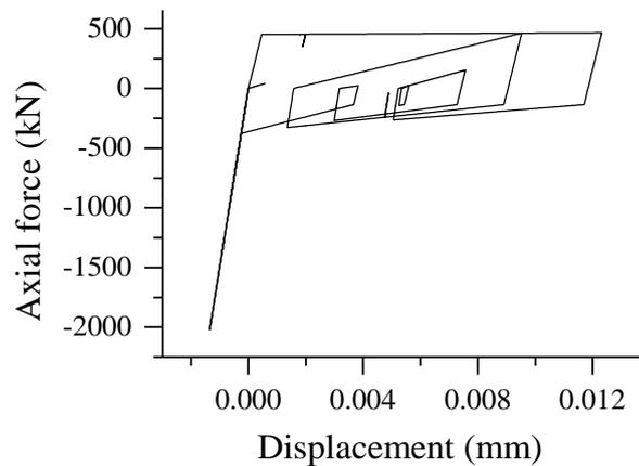
Figure 8. Axial stiffness hysteretic curve of the outside vertical element in the first floor subjected to the peak ground acceleration 400gal
