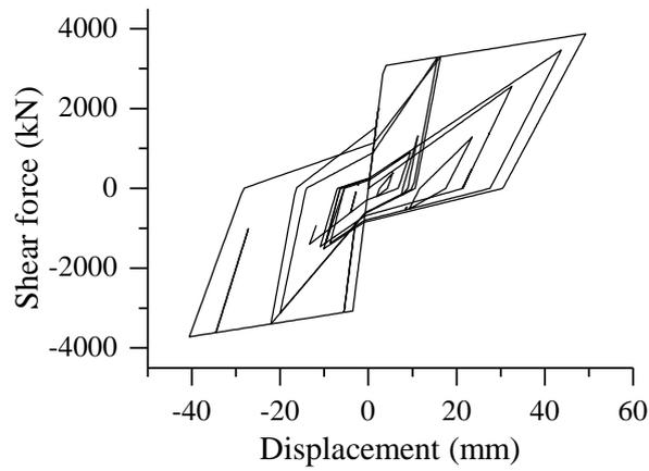
Figure 5. Shear hysteretic curve of the first floor subjected to the peak ground acceleration 220gal
