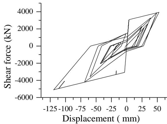
Figure 7. Shear hysteretic curve of the first floor subjected to the peak ground acceleration 400gal
