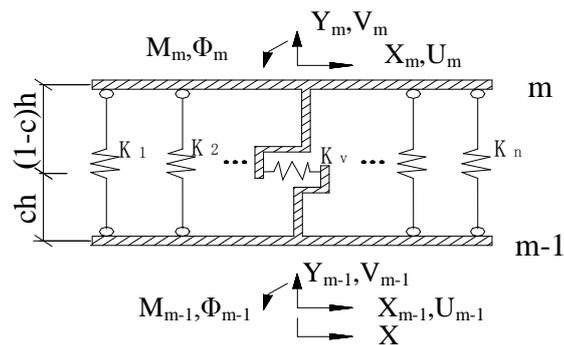
Figure 1. Multiple-vertical-line-element model
