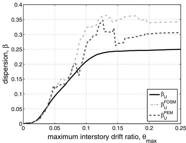
Figure 5 The values of  $\beta_U$  estimated using Monte Carlo simulation, FOSM and Rosenblueth's PEM given  $\theta_{\max}$
