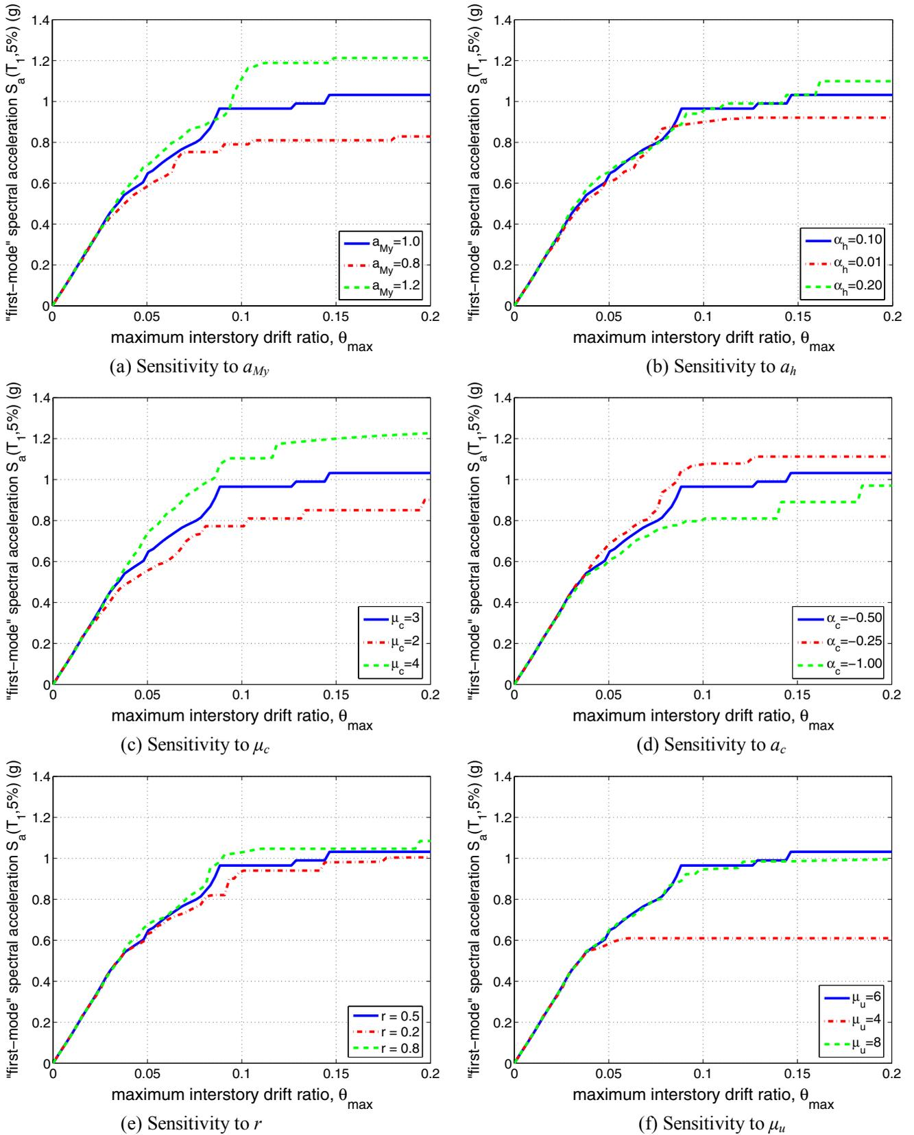
Figure 3 Sensitivity of the median IDA results to the beam-hinge backbone parameters
