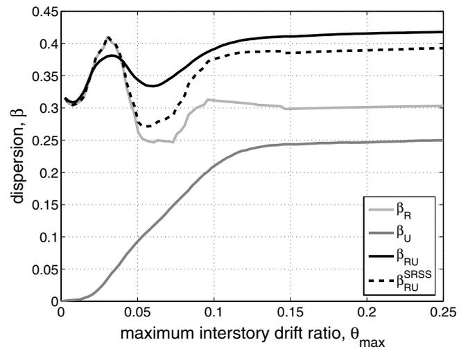
Figure 6 The values of  $\beta_U$ ,  $\beta_R$ ,  $\beta_{RU}$  compared against the SAC/FEMA approximation  $\beta_{RU}^{SRSS}$  given  $\theta_{\max}$
