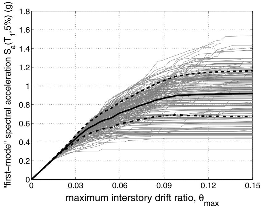
Figure 4 The 200 median IDAs shown against their mean and +/- one standard deviation curves
