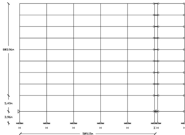
Figure 1 The LA9 steel moment-resisting frame
