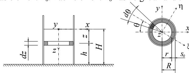
Figure 2. The sector of circular annulus (dark grey hatching) identified by the central angle  $\theta$  of the external torus of the grain (grey hatching)
