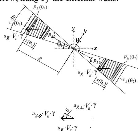
Figure 5. Vertical and horizontal actions operating on disk  $D$  and symmetrical elements  $E$  placed at different heights in the presence of additional horizontal and vertical acceleration
