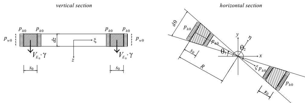
Figure 3. Vertical and horiz. actions operating on two symmetrical elements  $E_0$  under static conditions
