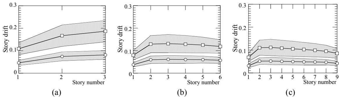
Figure 4. The mean and standard deviation of maximum story drift, (a) for 3-story frame, (b) for 6-story frame and (c) for 9-story frame
