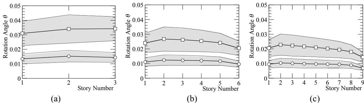
Figure 5. The mean and standard deviation of floor rotation angle (a) for 3-story frame, (b) for 6-story frame and (c) for 9-story frame.
