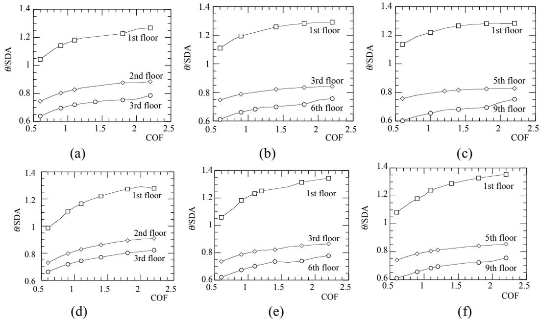
Figure 6. The ratio of rotation angle to story drift angle: (a) 3-story frame, (b) 6-story frame and (c) 9-story frame with  $A_0 = 600$  gal; (d) 3-story frame, (e) 6-story frame and (f) 9-story frame with  $A_0 = 1200$  gal.
