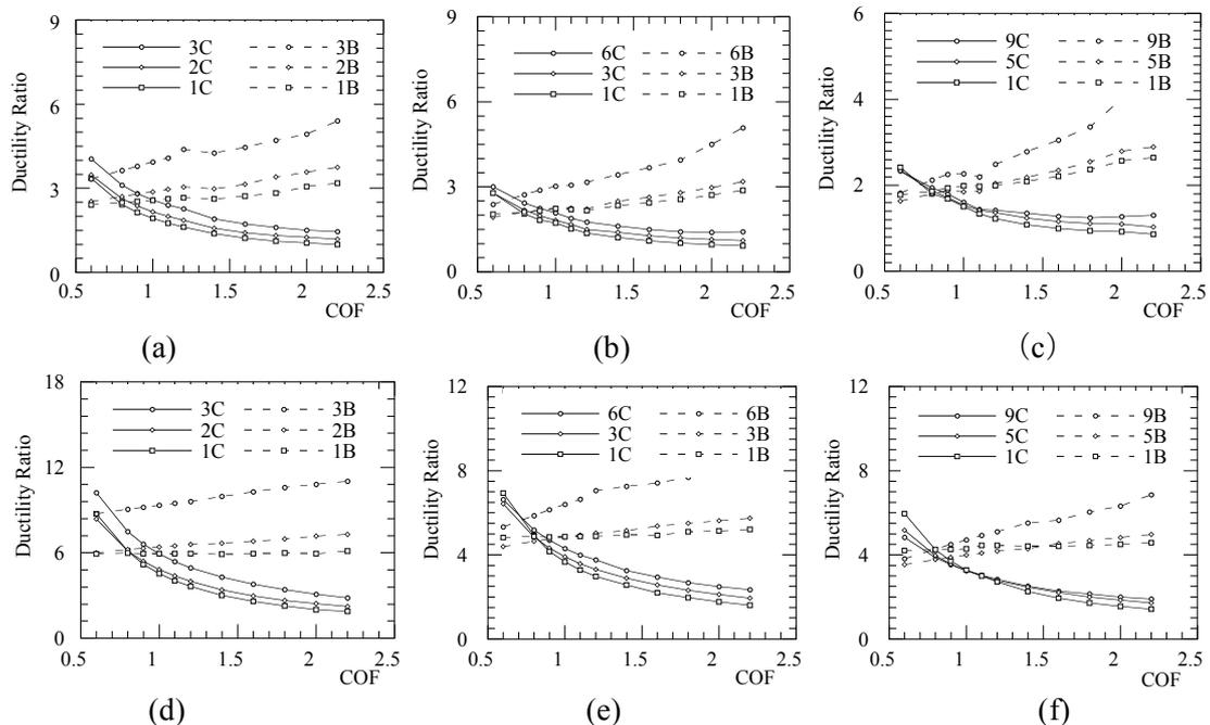
Figure 7. The effect of column over-design factor on the ductility ratio of columns and beams of frames: (a) 3-story frame, (b) 6-story frame and (c) 9-story frame for  $A_0 = 600$  gal; (d) 3-story frame, (e) 6-story frame and (f) 9-story frame for  $A_0 = 1200$  gal.
