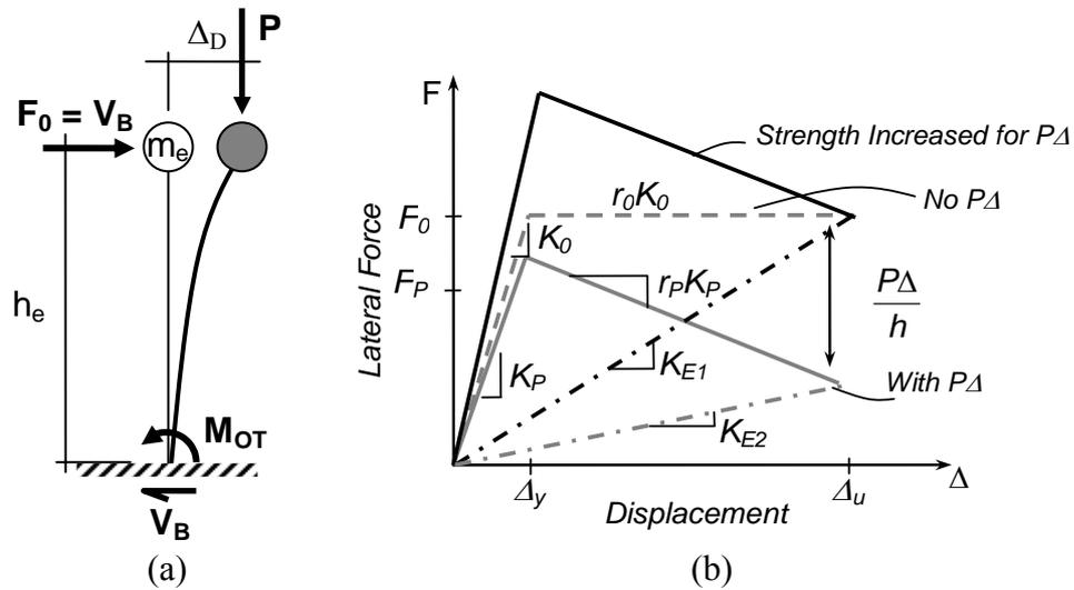
Figure 1. Effect of P- $\Delta$  on a Cantilever SDOF system (a) Structure and actions (b) Force-displacement response showing targeted effective stiffness
