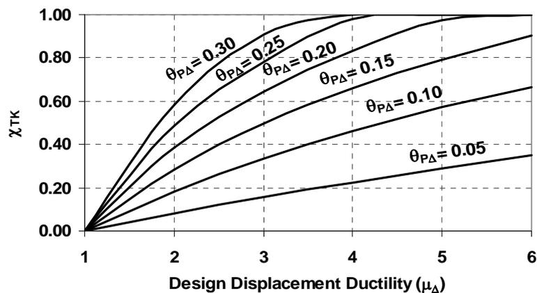
Figure 6. Design chart for  $\chi_{TK}$  to be used with DDBD
