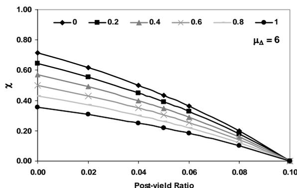
Figure 3. Parametric behaviour of  $\chi_{TK}$  as a function of post-yield stiffness ratio and Takeda reloading factor  $\beta$  for values 0 to 1.0 shown by each separate line ( $\theta_{P\Delta} = 0.10$ ).
