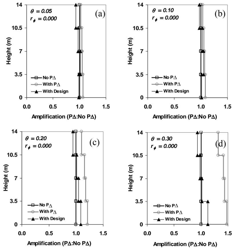
Figure 4. Elasto-plastic (EP) four-storey frame model drift amplification profiles at ground motion intensity 1.0x design ( $\mu_{\Delta} = 1.56$ ) and  $r_{\phi} = 0.0\%$ .
