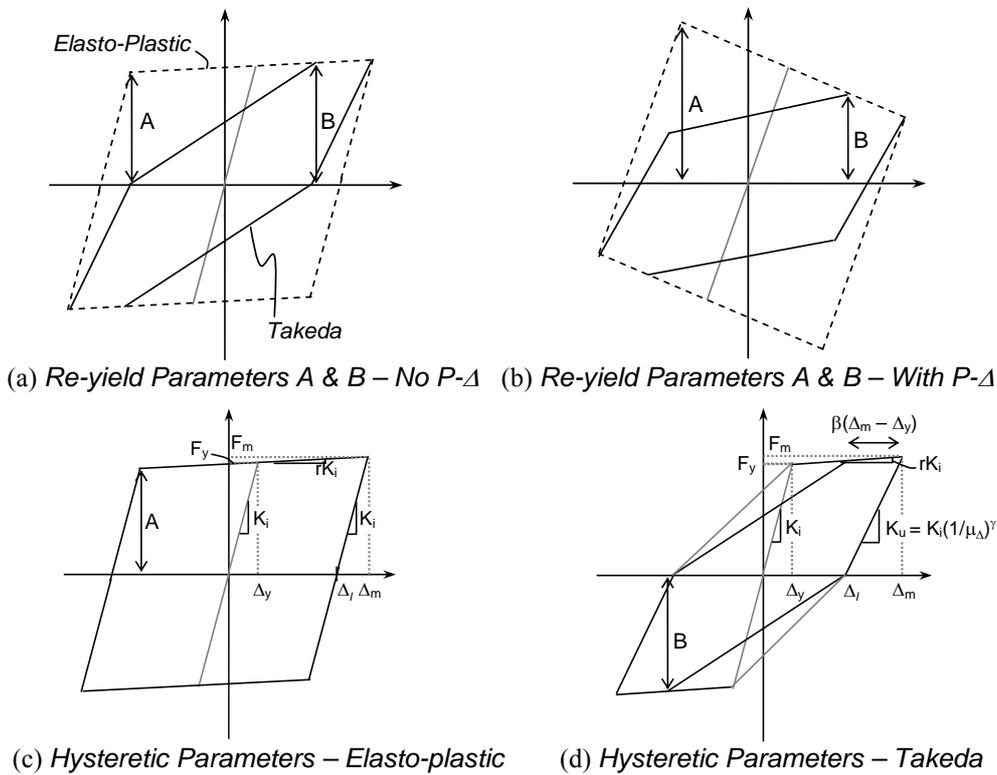
Figure 2. Hysteretic parameters used for derivation of  $\chi$
