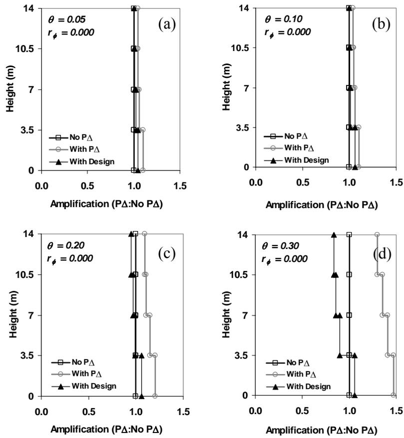
Figure 5. Takeda (TK) four-storey frame model drift amplification profiles at ground motion intensity 1.0x design ( $\mu_{\Delta} = 2.40$ ) and  $r_{\phi} = 0.0\%$
