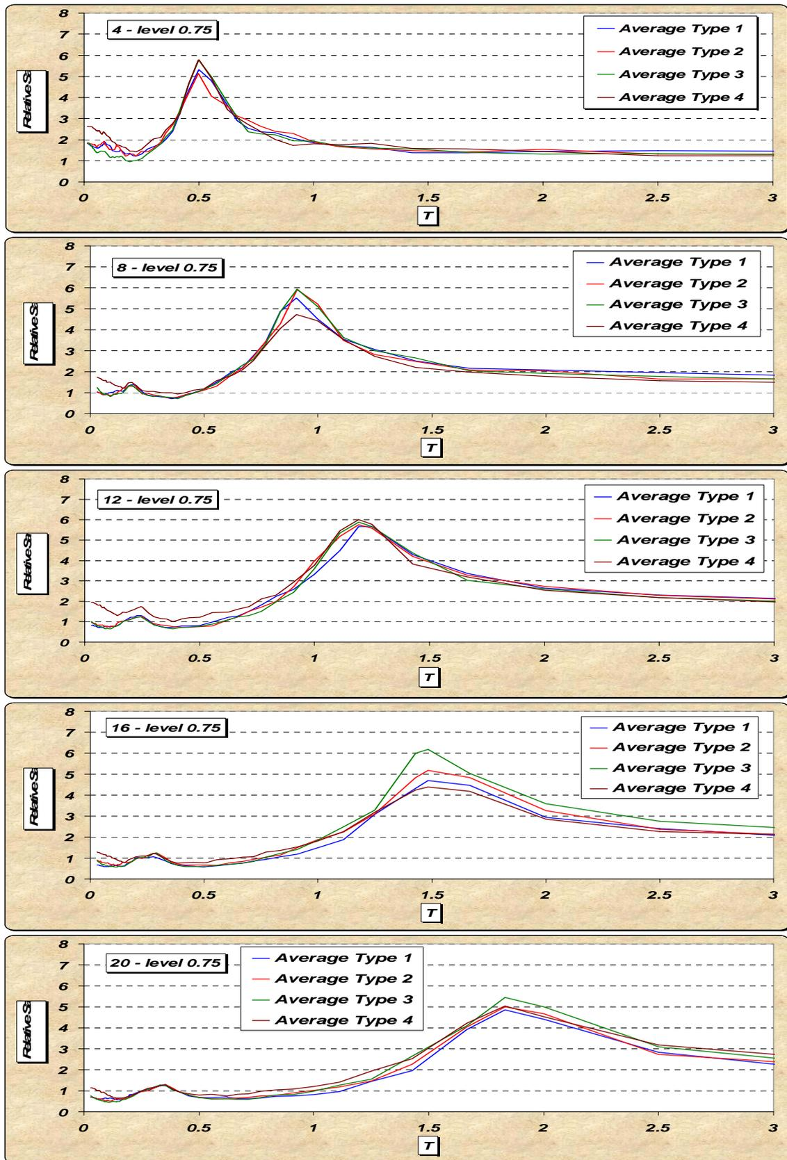
Figure 3. Comparison of average of relative ARSF for each one of the soil types and at the level of 0.75 of 4, 8, 12, 16 and 20 story models
