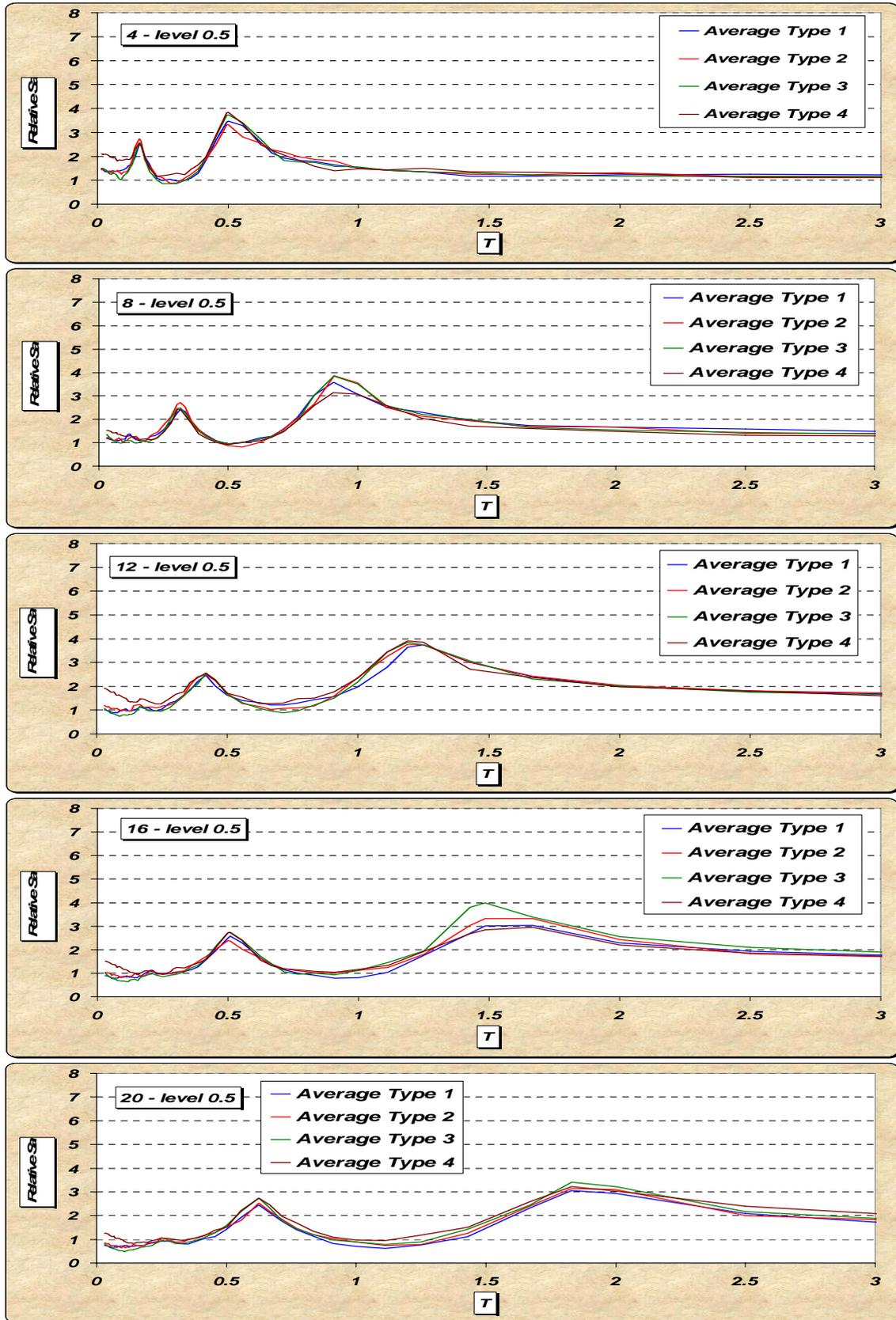
Figure 2. Comparison of average of relative ARSF for each one of the soil types and at the level of 0.5 of 4, 8, 12, 16 and 20 story models
