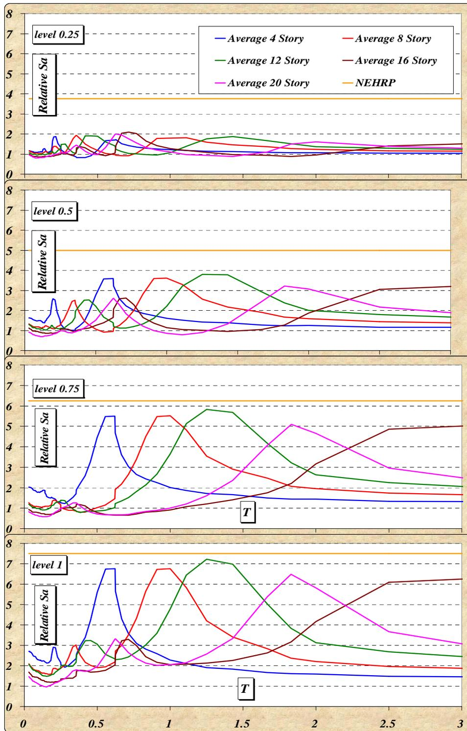
Figure 5. Comparison of ratio of average of ARSF for each one of models and the NEHRP (2003) procedure at the levels of 0.25, 0.5, 0.75 and 1
