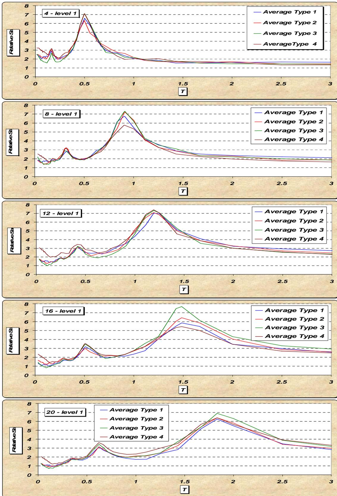
Figure 4. Comparison of average of relative ARSF for each one of the soil types and at the level of 1 of 4, 8, 12, 16 and 20 story models
