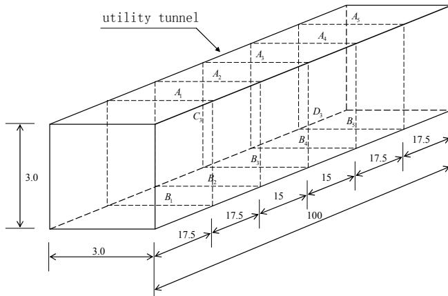
Fig. 5 Typical Output point on the utility tunnel
