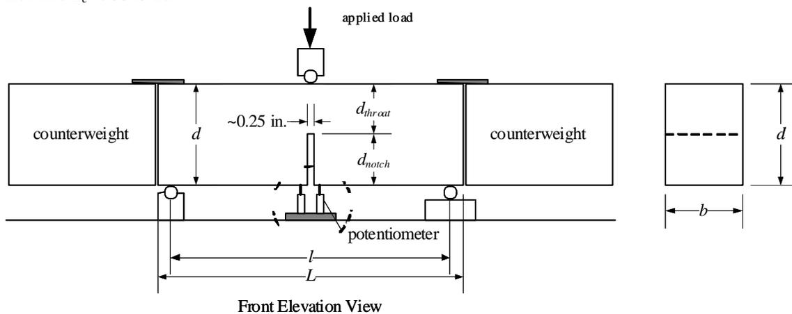
Figure 1. Fracture energy test at University of Washington (Martin et al. 2007)
