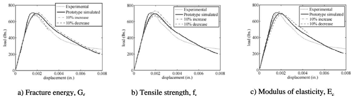
Figure 8. Variation with uncertainty in measurement of material parameters
