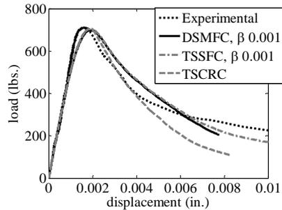
Figure 4. Variation with different smeared crack models
