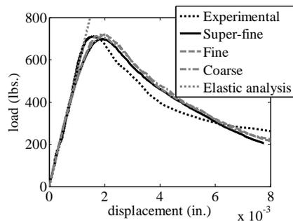
Figure 2. Simulation of fracture energy test
