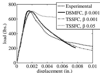
Figure 5. Variation with shear retention factor
