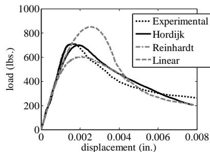
Figure 3. Variation with concrete tensile post-peak softening curve
