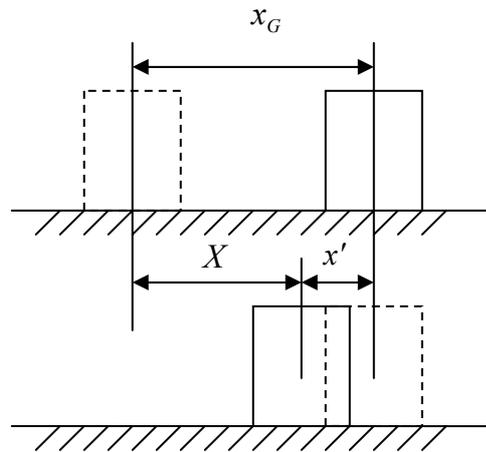
Figure 3.4 Displacement in sliding
