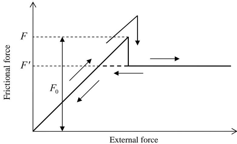
Figure 3.2 Relation between frictional force and external force
