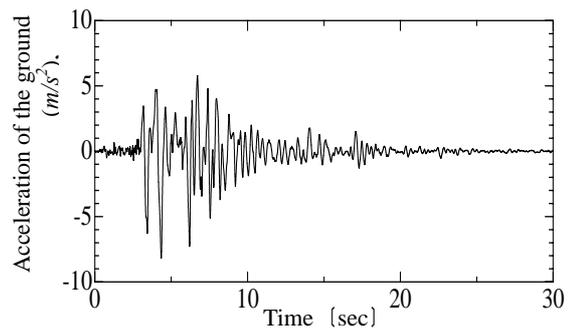
Figure 4.7 Ground acceleration record at 1995 Southern Hyogo Earthquake
