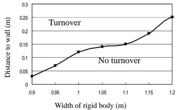
Figure 4.6 Relation between width of rigid body and distance to wall
