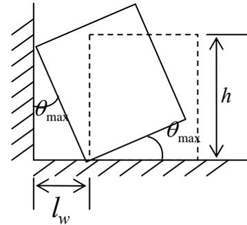
Figure 3.7 Collision of rigid body with wall
