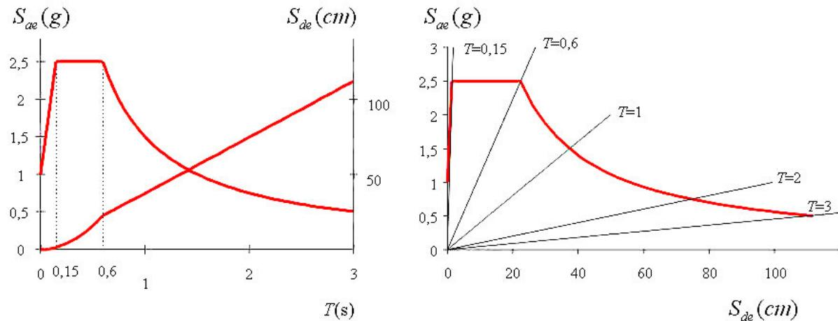
Figure 1 Acceleration spectrum (N2 method)
