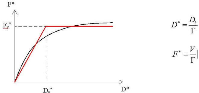
Figure 3 Idealization of force – displacement relation
