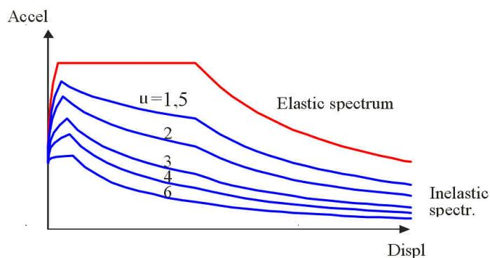
Figure 2 Inelastic spectrum
