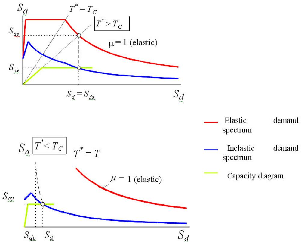
Figure 4 Elastic and demand spectrum in relation with capacity diagram
