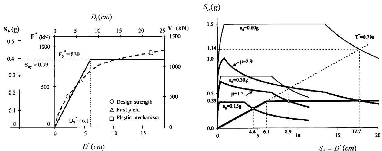
Figure 8 Pushover curve and capacity diagram (left part of the picture); demand spectrum for 3 different ground accelerations and capacity diagram (right part of the picture)
