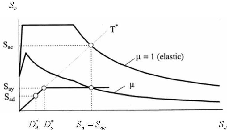
Figure 6 Demand and capacity spectrum
