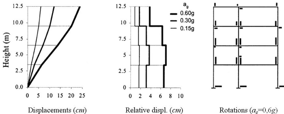
Figure 9 Displacements, relative displacements and rotations of frame
