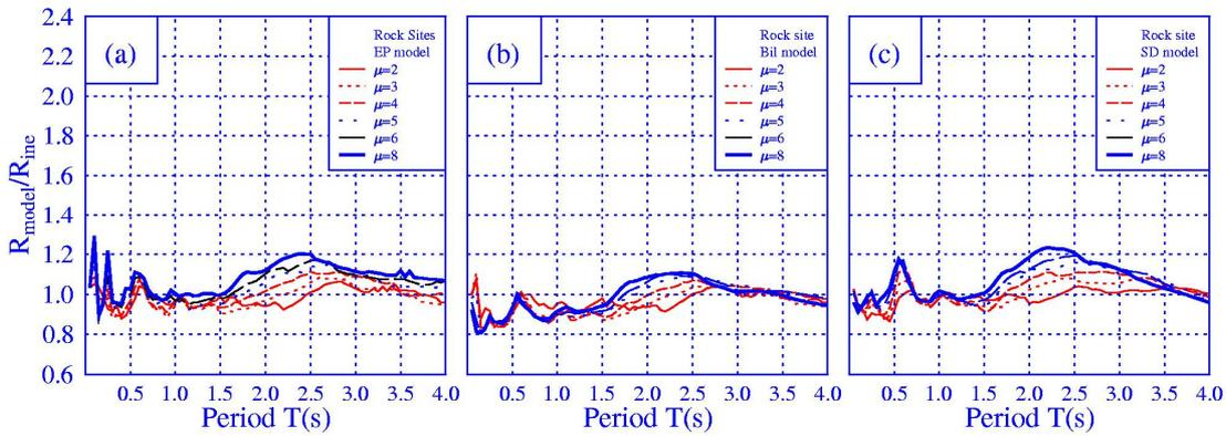
Figure 7 Comparisons of the R-factor ratios of the approximate to exact R-factors for  $\mu=2, 3, 4, 5, 6,$  and  $8$  on rock sites for the three hysteretic models calculated from the new model (Eqn.6.3) (EP: perfectly elastic-plastic model; Bil: bilinear model; SD: stiffness degrading model).
