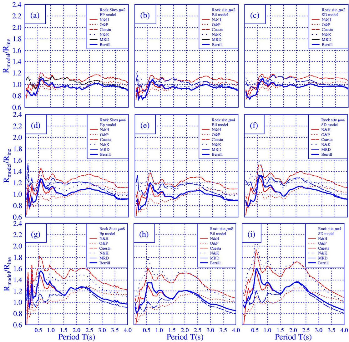
Figure 1 Comparisons of the R-factor ratios of the approximate to the exact R factors for  $\mu=2, 4,$  and  $8$  on rock sites for the three hysteretic model (N&H: the Newmark & Hall model; Ordaz: the Ordaz and Perez-Rocha model; Cuesta: the Cuesta et al model; N&K: the Nassar & Krawinkler model; MRD: the Miranda model; Berrill: the Berrill et al model, and EP: perfectly elastic-plastic model; Bil: bilinear model; SD: stiffness degrading model).
