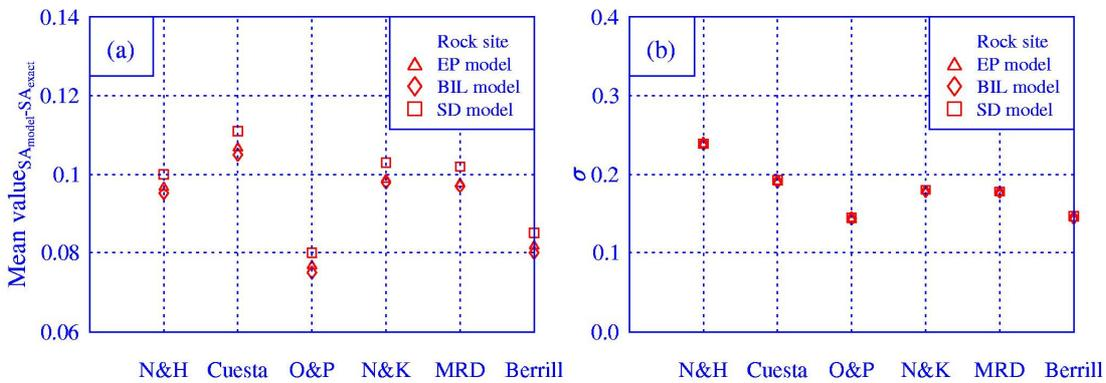
Figure 5 Comparisons of the mean values (a) and standard deviations (b) of the difference between the approximate and exact inelastic spectra for the existing 6 R-factor models on rock sites (EP: perfectly elastic-plastic model; Bil: bilinear model; SD: stiffness degrading model).
