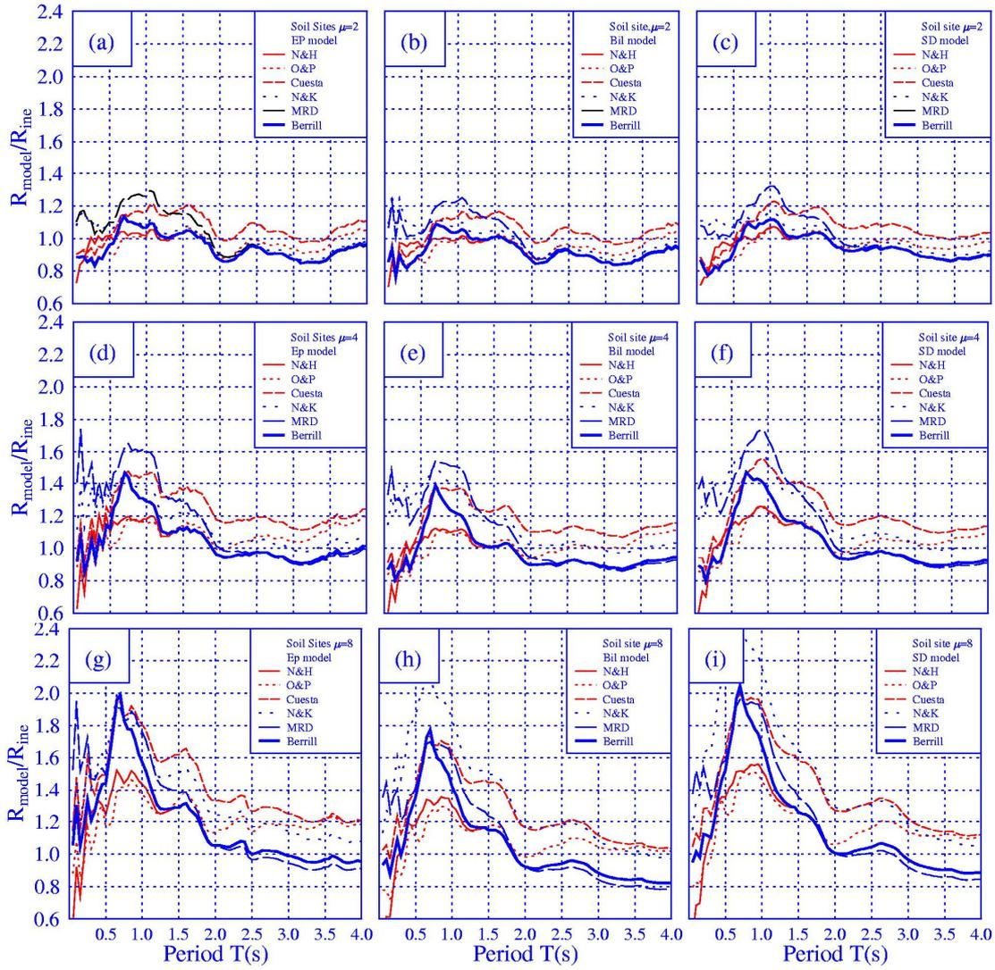
Figure 3 Comparisons the R-factor ratios of the approximate to the exact R factors for  $\mu=2, 4,$  and  $8$  on soil sites for the three hysteretic models (the meaning of these labels shows in the caption of Figure 1)
