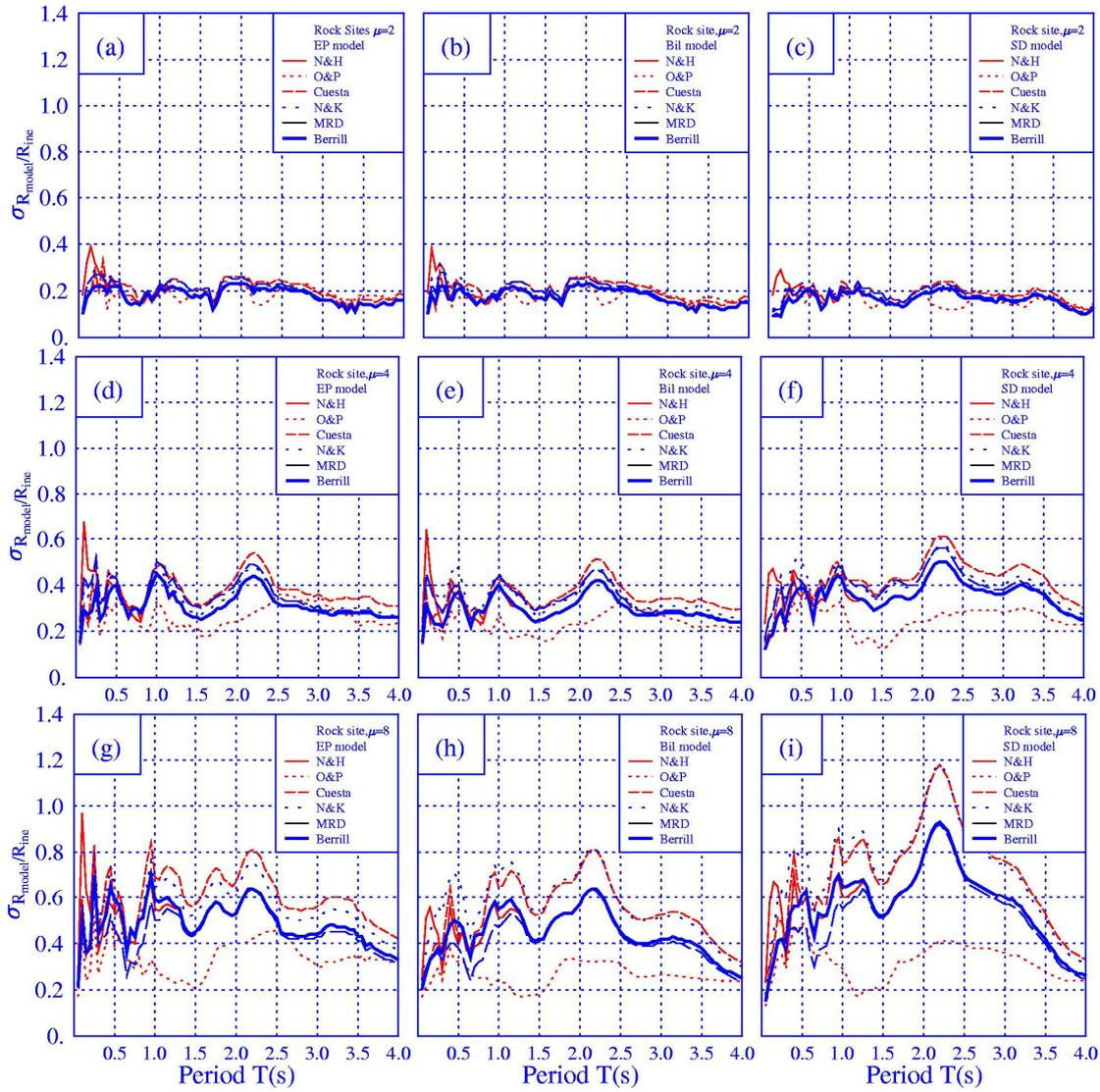
Figure 2 Comparisons of standard deviations of the R-factor ratios for  $\mu=2, 4,$  and  $8$  on rock sites for the three hysteretic models (the meaning of these labels shows in the caption of Figure 1).
