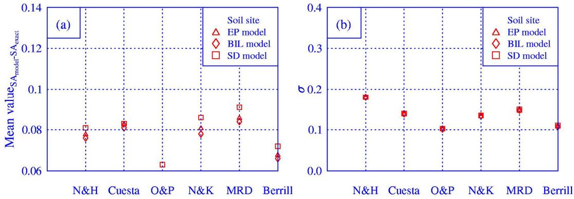
Figure 6 Comparisons of the mean values (a) and standard deviations (b) of the difference between the approximate and exact inelastic spectra for the existing 6 R-factor models on soil sites (EP: perfectly elastic-plastic model; Bil: bilinear model; SD: stiffness degrading model).
