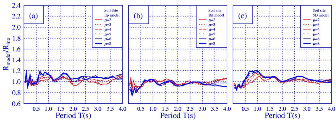
Figure 8 Comparisons of the R-factor ratios of the approximate to exact R-factors for  $\mu=2, 3, 4, 5, 6,$  and  $8$  on soil sites for the three hysteretic models calculated from the new model (Eqn.6.4) (EP: perfectly elastic-plastic model; Bil: bilinear model; SD: stiffness degrading model).
