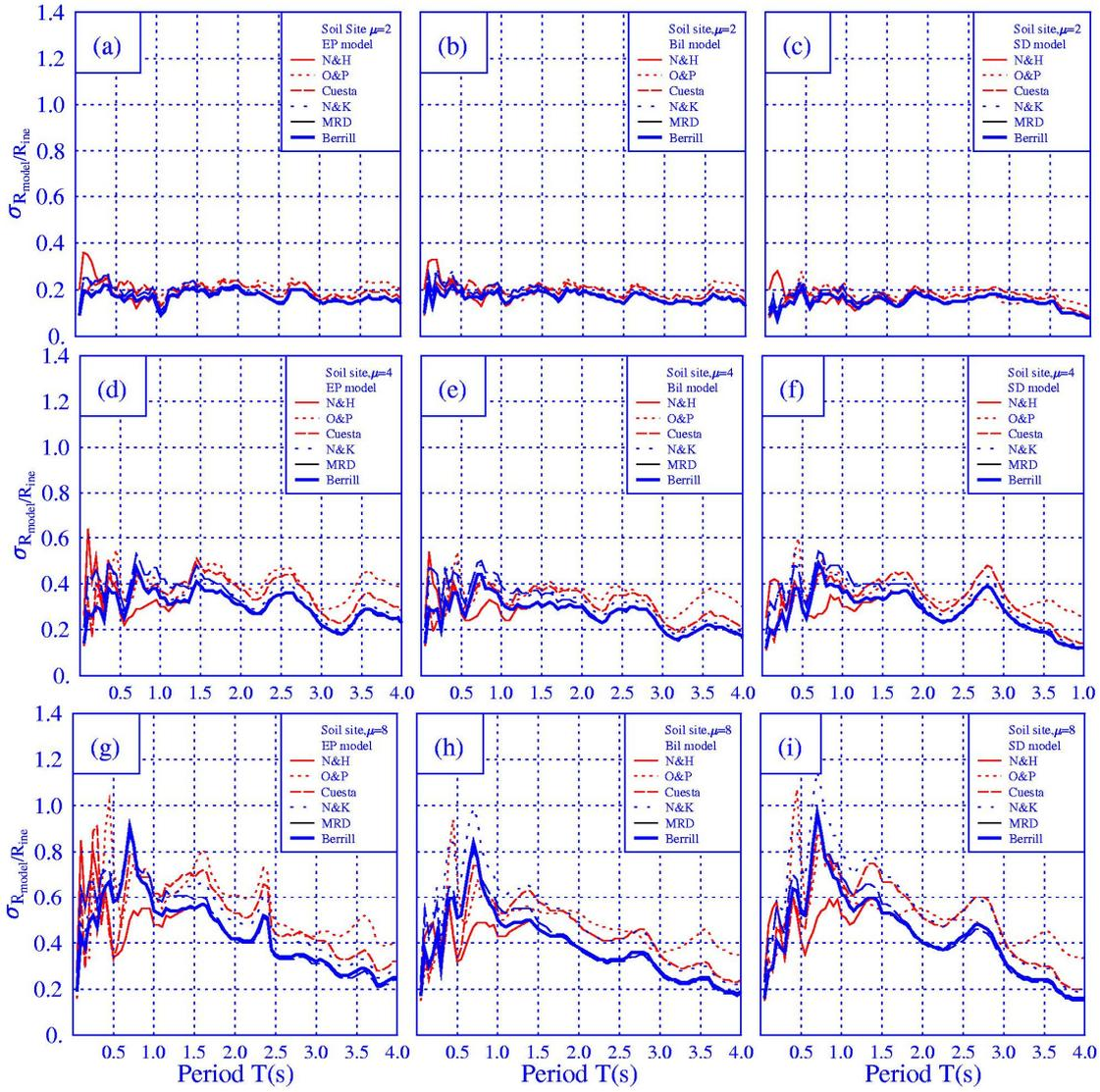
Figure 4 Comparisons of standard deviations of the R-factor ratios for  $\mu=2, 4,$  and  $8$  on soil sites for the hysteretic models (the meaning of these labels shows in the caption of Figure 1).
