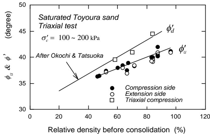
Figure 1 Variety of friction angle with relative density
