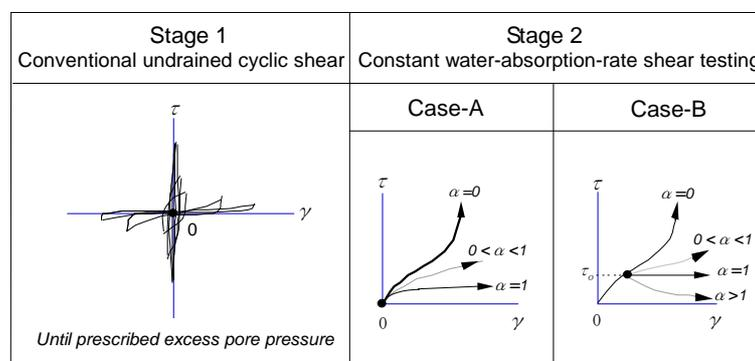
Figure 2 Test program of constant water-absorption-rate shear testing
