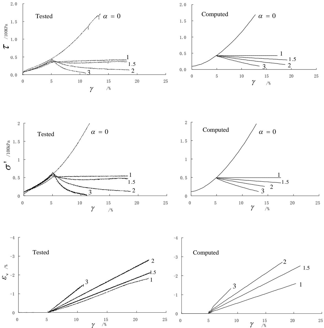
Figure 4 Results of test and simulation for Case B
