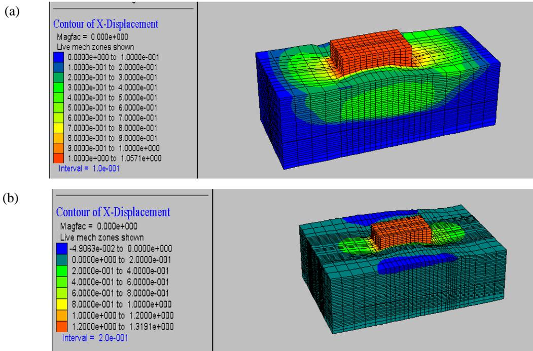
Figure 5. 3D Horizontal Displacement Contours (E-W) for SFTS Moving East: (a) NSR Model, (b) JG Model
