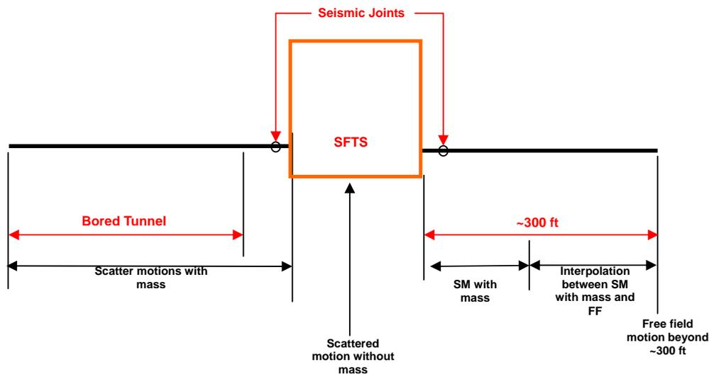
Figure 8. Schematic Showing Transition of Scatter Motions Near the SFTS to Free-Field Motions along TBT
