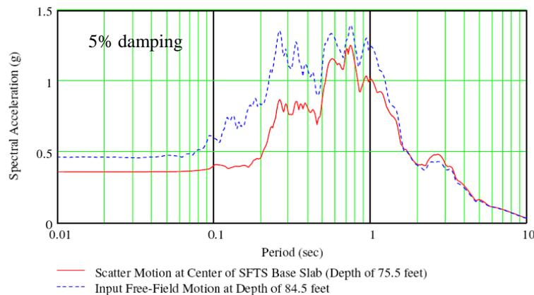
Figure 7. Comparison of Scatter Motion and SASSI Input Motion spectra in X Direction – Capitola Motion
