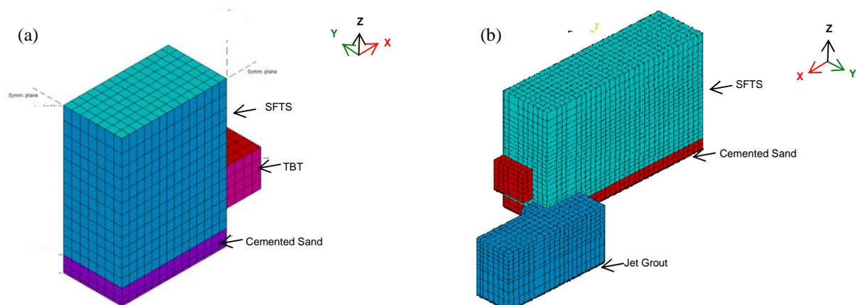
Figure 2. SASSI models for the SFTS: (a) NSR Model, and (b) JG Model
