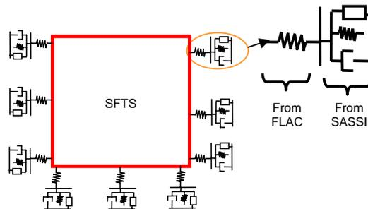
Figure 1. Schematic Showing Soil-Interaction Analysis Approach for the SFTS
