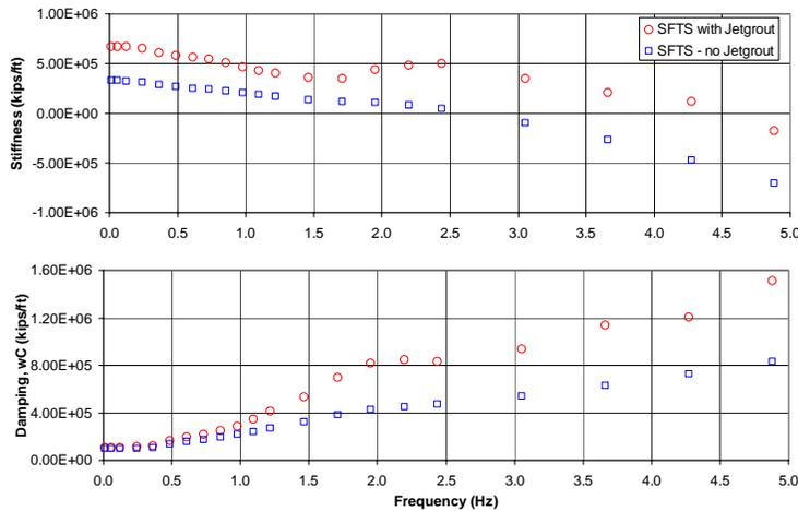
Figure 4. Example of Impedance Results: Stiffness and Damping in X Direction for NSR and JG Models
