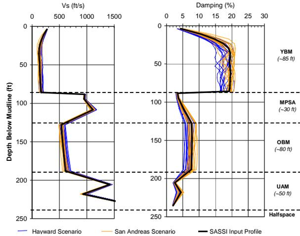
Figure 3. Development of SASSI Input Soil Properties
