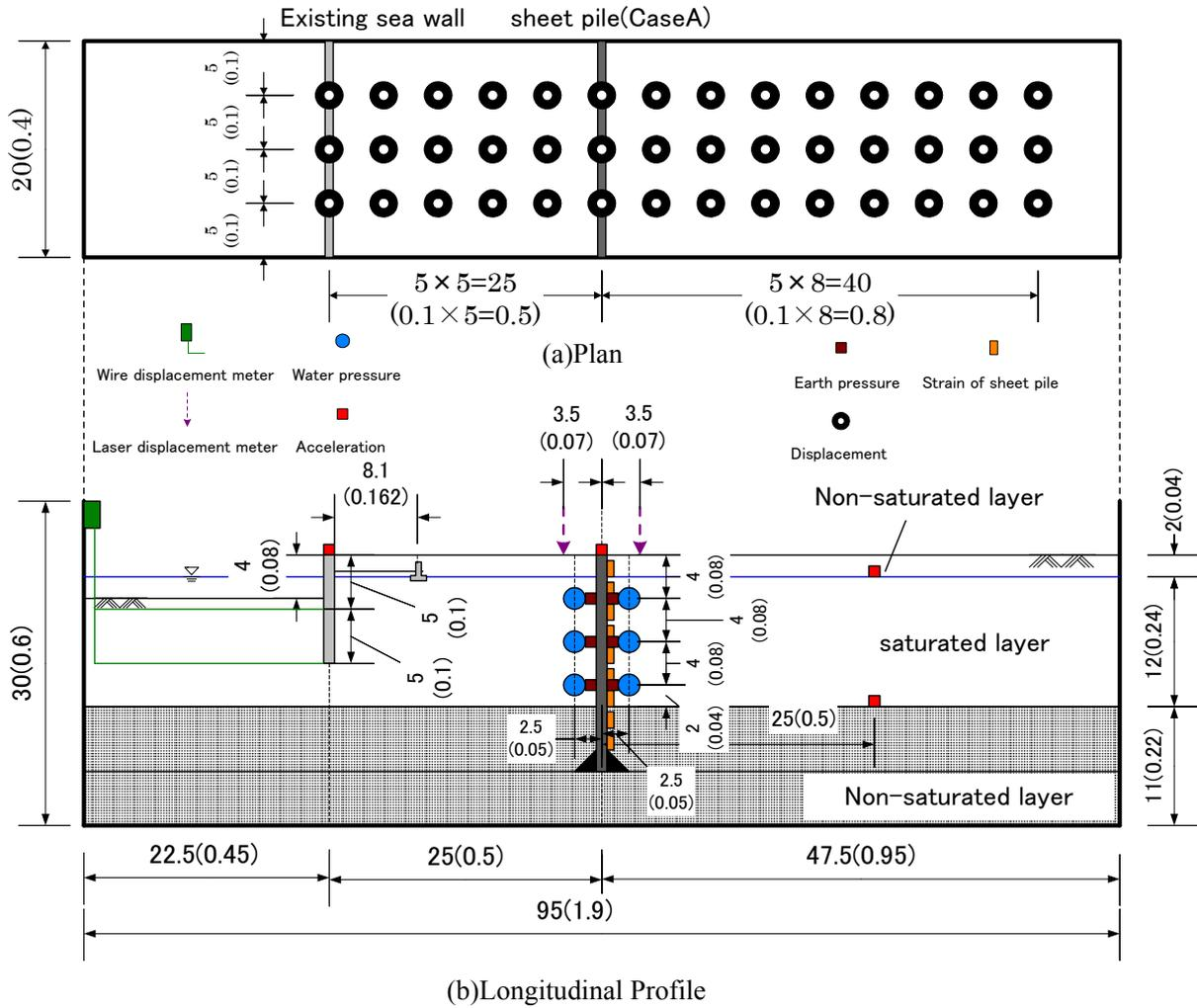
Figure 2 Locations of measurement instruments
