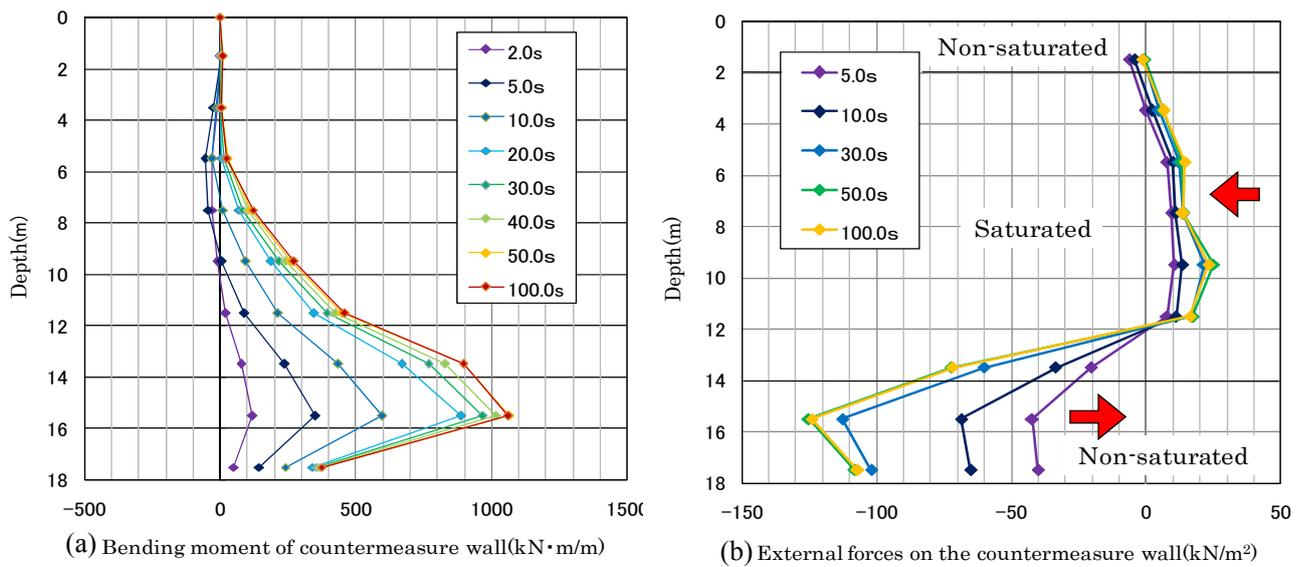
Figure 4 Bending moment of the countermeasure wall and external forces (Case B)
