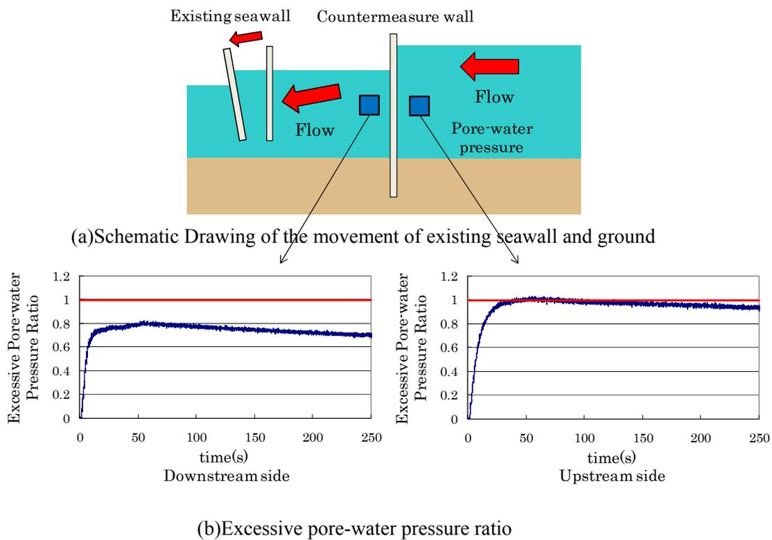
Figure5 Movement of the existing seawall and ground, and excessive pore-water pressure ratio
