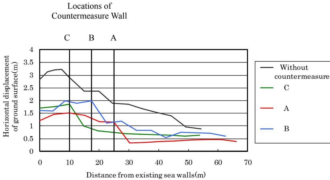
Figure 3 The Effectiveness of countermeasure walls to reduce the ground displacement in horizontal direction
