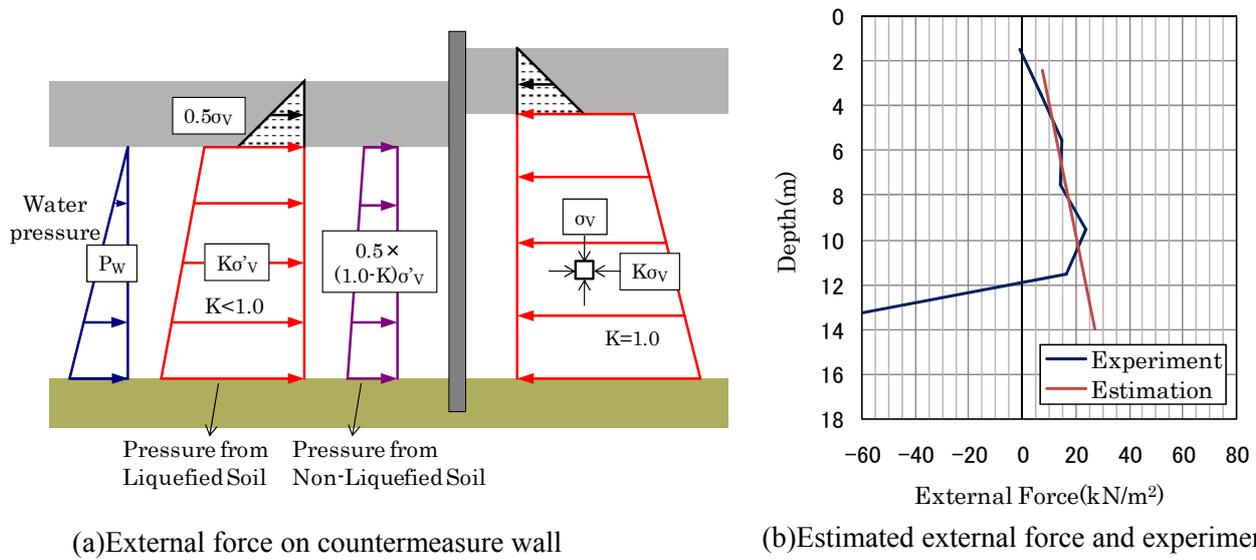
Figure 6 Estimation of external forces on the countermeasure walls
