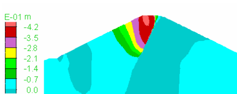
Figure 12a Vertical displacement profile after earthquake (ICD)
