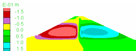
Figure 5a Horizontal displacement contours at the end of construction (VCD)
