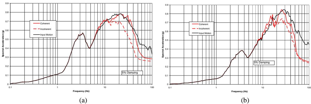
Figure 8 Comparison of the (a) Horizontal and (b) Vertical Response Spectra of Input Motion and Foundation Response Motion at Grade Level
