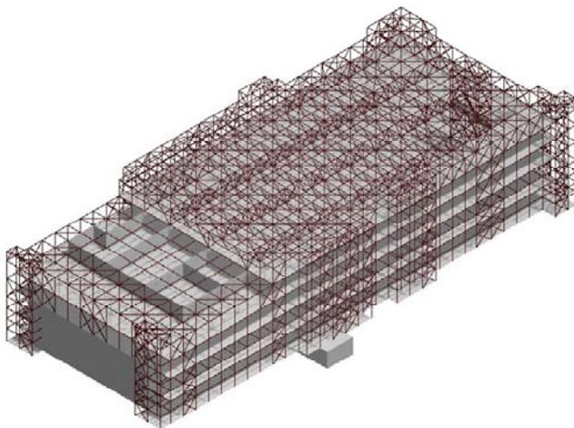
Figure 3 SASSI2000 Model of the Vitrification Building
