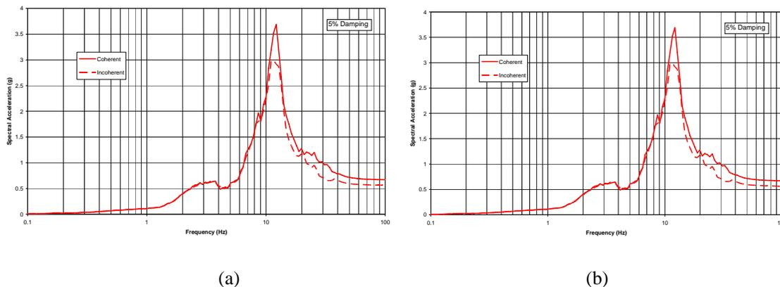
Figure 9 Comparison of the (a) Horizontal and (b) Vertical Response Spectra at the Elevation 68 ft
