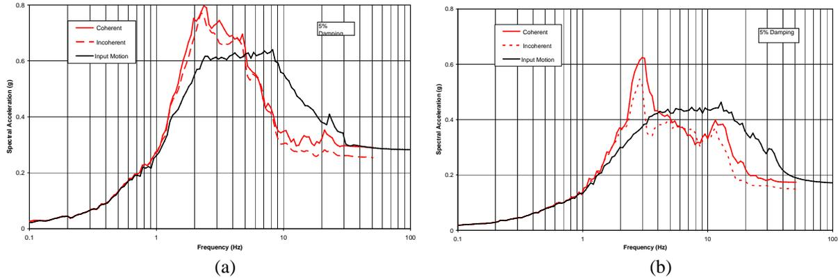
Figure 5 Comparison of the (a) Horizontal and (b) Vertical Response Spectra of Input Motion and Foundation Response Motion at the Grade Level
