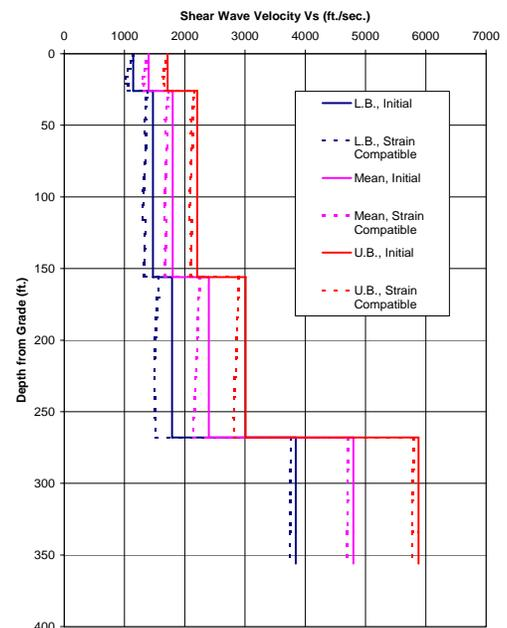
Figure 4 Shear Wave velocity profile at Location of the Vitrification Facility
