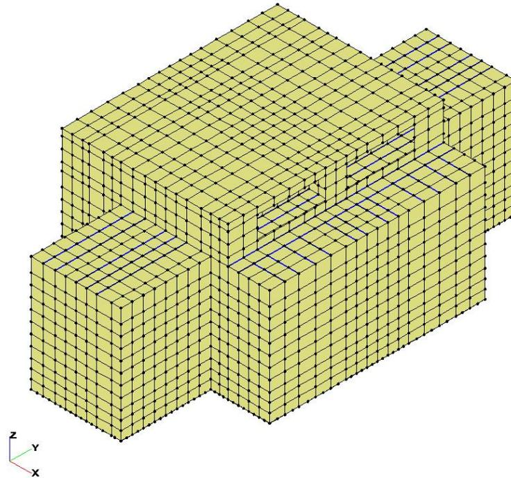
Figure 7 SASSI2000 Model of the Diesel Generator Building
