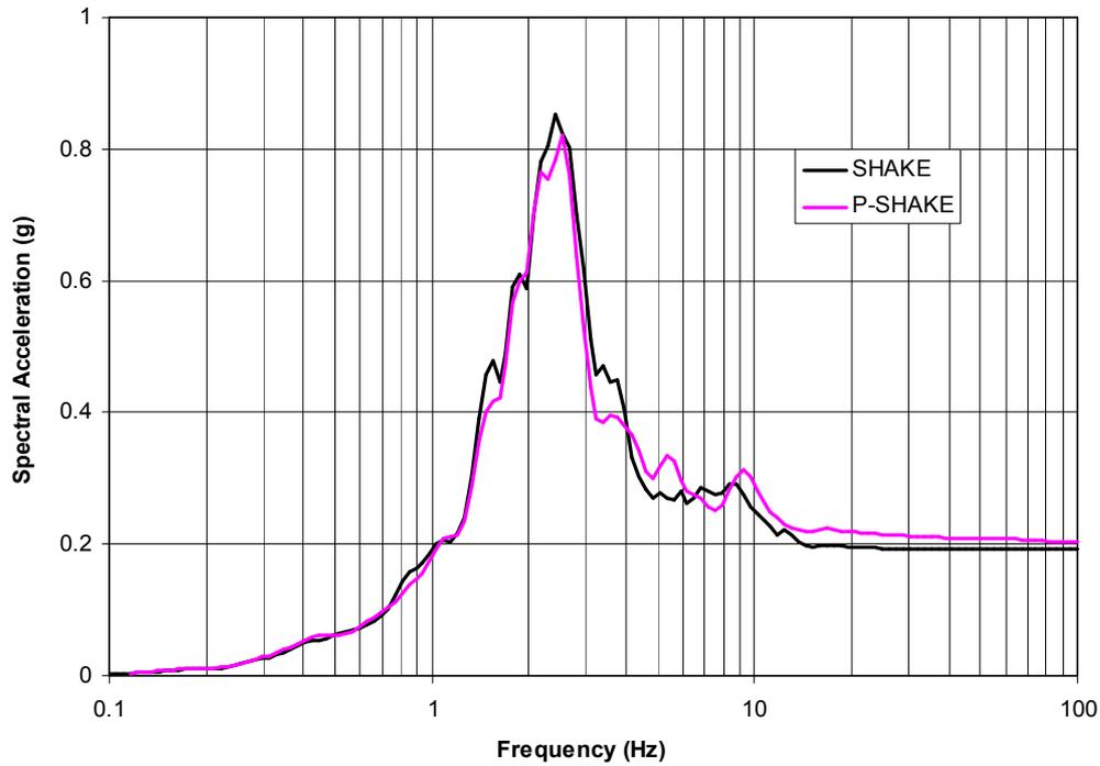
Figure 7 Comparison of 5% Damped Acceleration Response Spectra at Ground Surface
