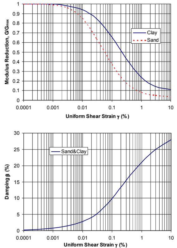
Figure 3 Modulus Degradation and Damping Relations vs. Shear Strains
