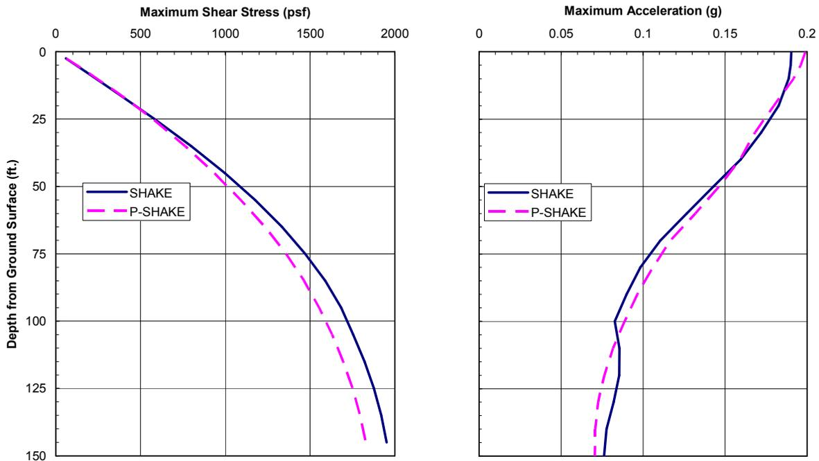
Figure 6 Comparison of Maximum Shear Stress and Maximum Acceleration Profiles
