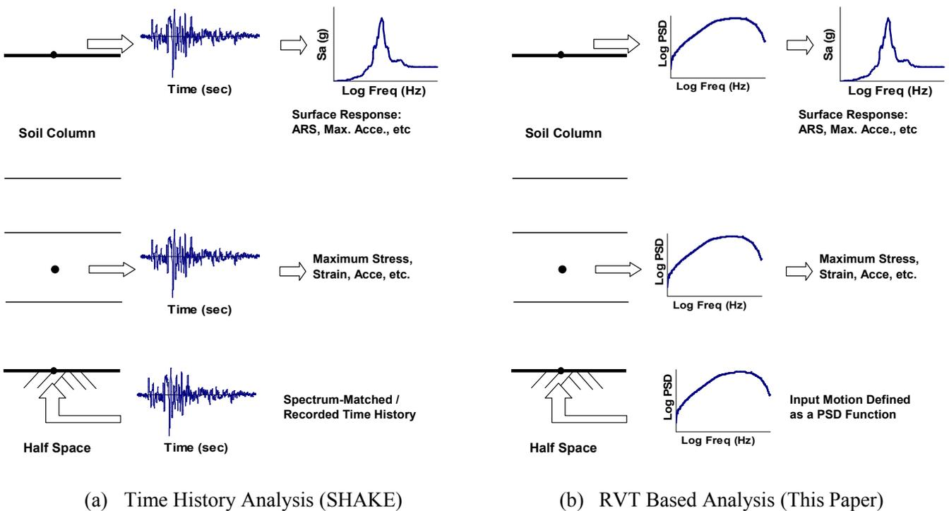
Figure 1 Different Approaches for Site Response Analysis
