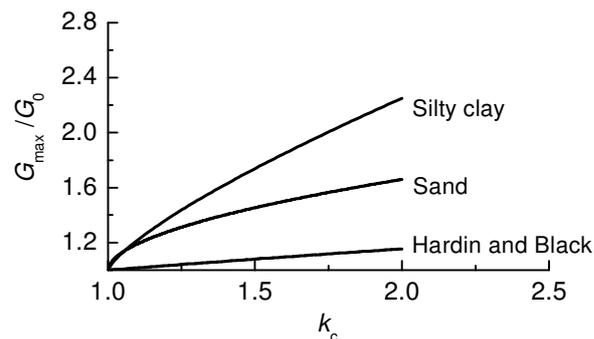
Figure 5 Comparison of  $G_{\max}/G_0-k_c$  for three formulas
