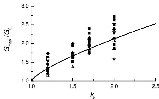
Figure 2 Comparison between the presented formula and test data of silty clay
