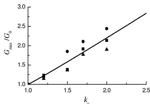
Figure 3 Comparison between the presented formula and test data of silt
