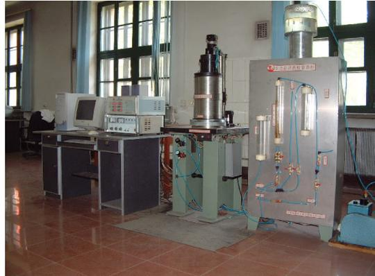
Figure 1 The resonant column device used for tests
