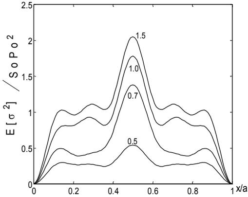
Figure (3) - The most probable stress for the different ratios of width to length
