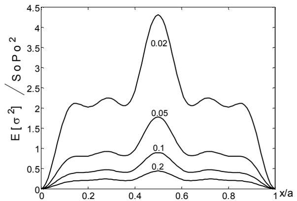
Figure (8) The most probable stress for the different amount of damping ratio
