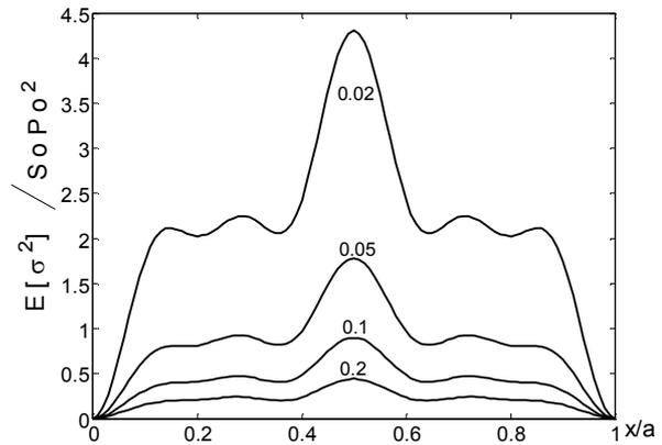
Figure (10)- The most probable stress for the different amount of bed hardening  $N/m/m^2$
