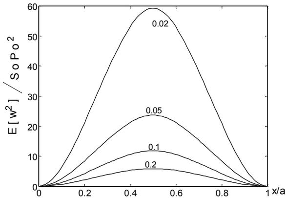
Figure (9) - The most probable deflection for the different amount of bed hardening  $N/m/m^2$
