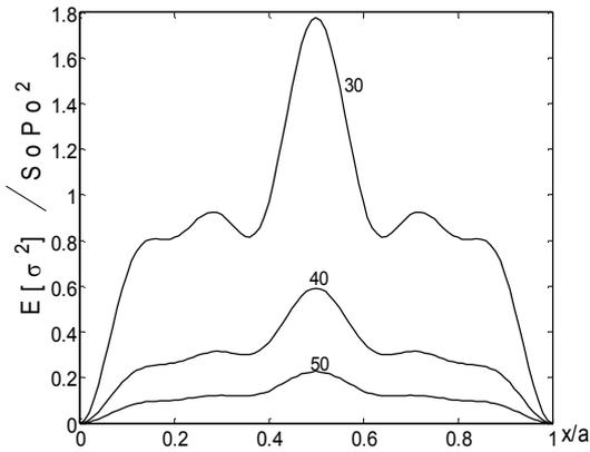
Figure (5) - The most probable stress for the different foundation thickness (cm)
