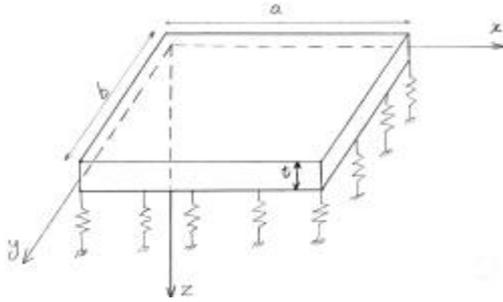
Fig. 1- Schematic of the foundation on the elastic bed figure
