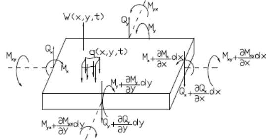
Fig. 2- The element of a foundation in dimension of dx, dy under random loading of external load and internal forces
