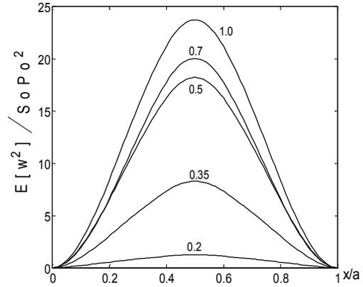
Figure (4) - The most probable deflection for the different ratios of width to length
