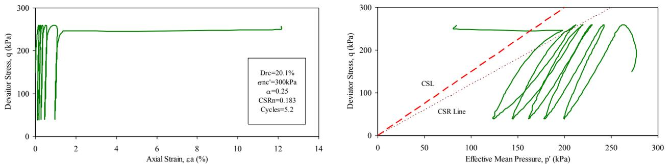
Figure 2 Cyclic behavior of sand ( $D_{rc}=20\%$ ,  $\sigma_{nc}'=300\text{kPa}$ ,  $\alpha=0.25$ )
