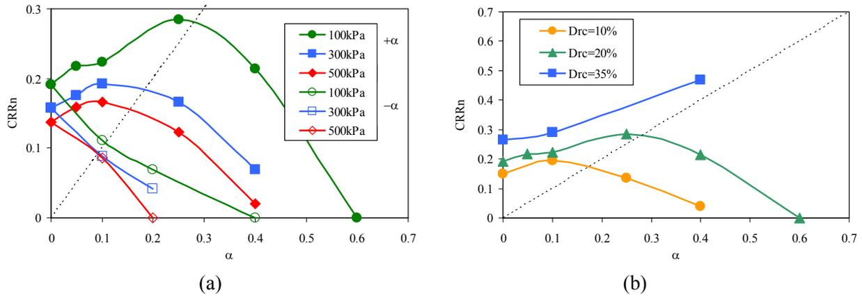
Figure 4  $CRR_n$  versus  $\alpha$  at various  $\sigma_{nc}'$  and  $D_{rc}$  values
