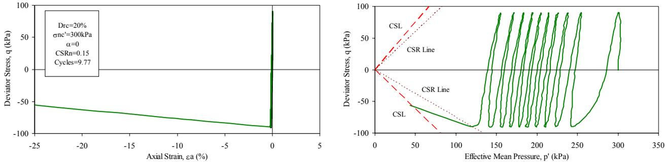
Figure 1 Cyclic behavior of sand ( $D_{rc}=20\%$ ,  $\sigma_{nc}'=300\text{kPa}$ ,  $\alpha=0$ )
