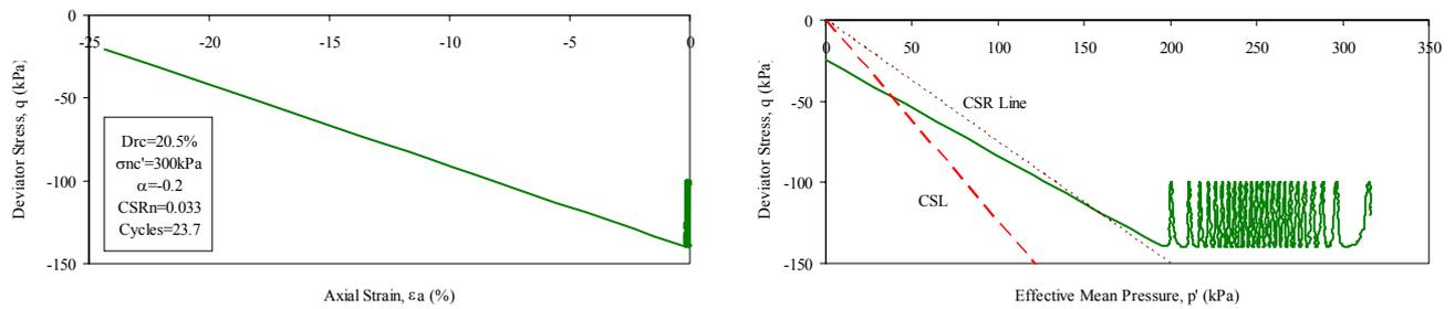
Figure 3 Cyclic behavior of sand ( $D_{rc}=20\%$ ,  $\sigma'_{nc}=300\text{kPa}$ ,  $\alpha=-0.2$ )
