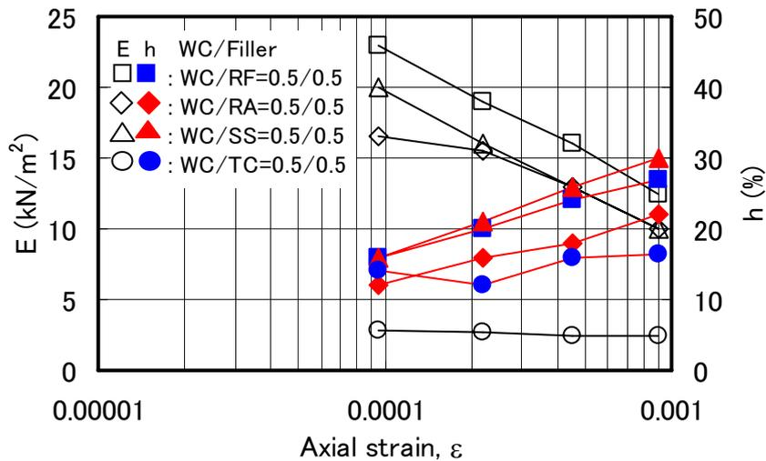
Figure 5 Strain dependency of  $E$  &  $h$  in case 3
