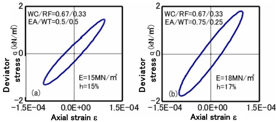
Figure 3 The stress-strain relationship in case 1
