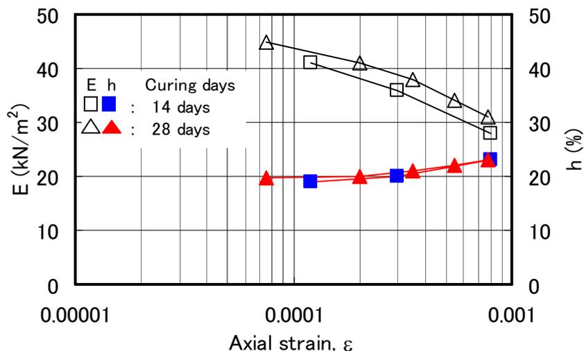
Figure 6 Strain dependency of  $E$  &  $h$  in case 4
