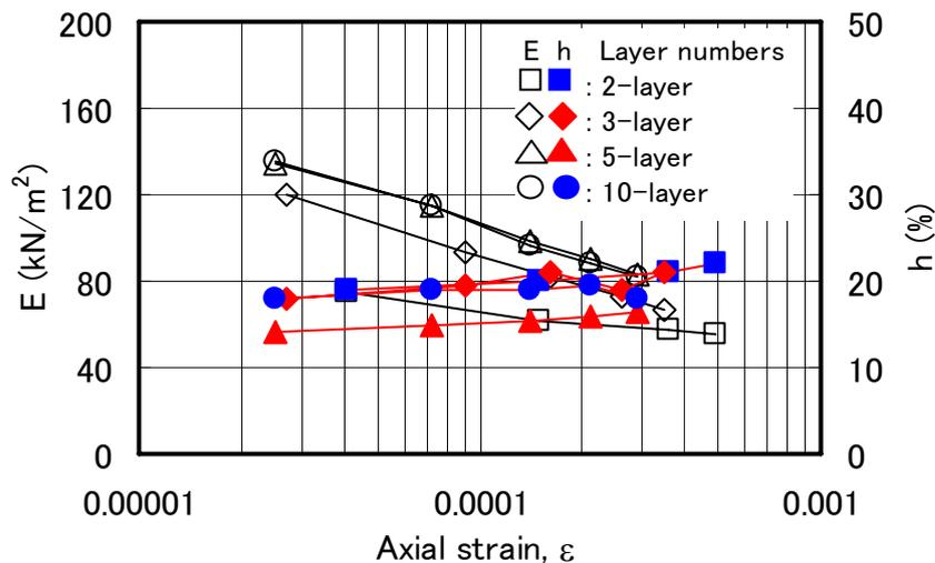
Figure 7 Strain dependency of  $E$  &  $h$  in case 5
