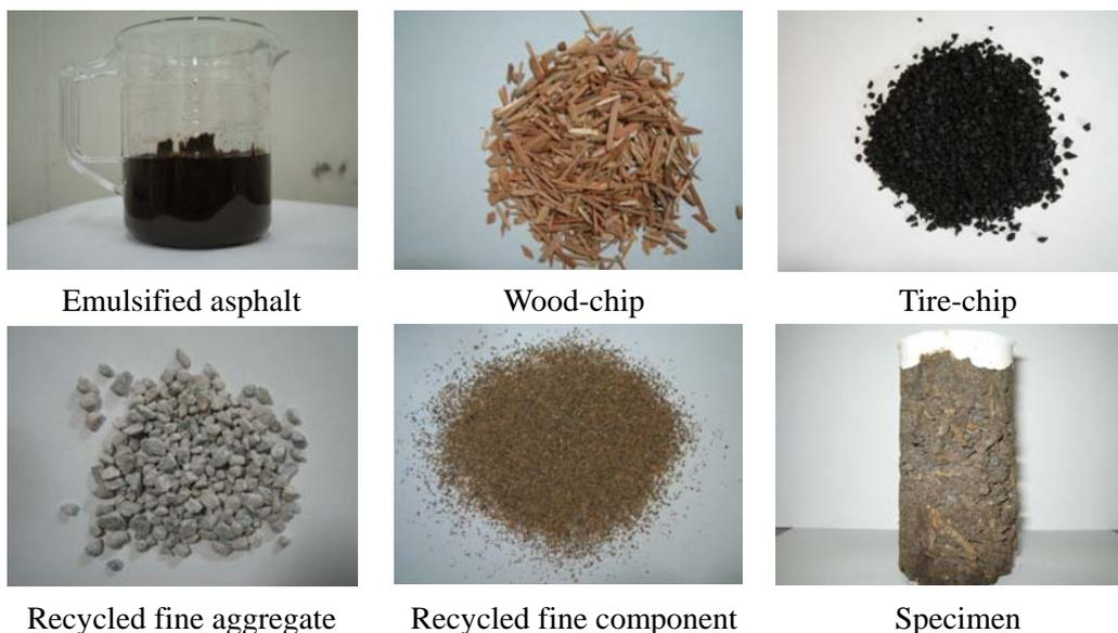
Photo 1. Materials used for manufacturing the plant-base vibration-damping block.
