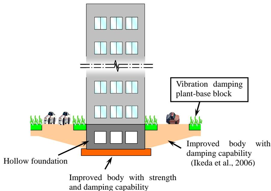
Figure 1 Concept of the proposed composite foundation
