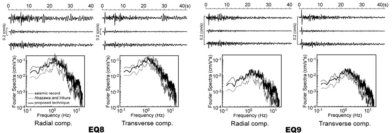
Fig.6 Examples of velocity waveforms (top: seismic record, middle: (Akazawa and Irikura, 2007) procedure, bottom: proposed technique) and velocity Fourier spectra re-created for events used in Section 5.2.
