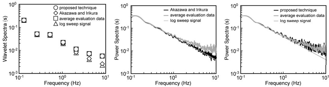
Fig.3 Obtained wavelet spectra (left), power spectra for Akazawa and Irikura (2007) procedure (center) and power spectra for proposed technique (right).
