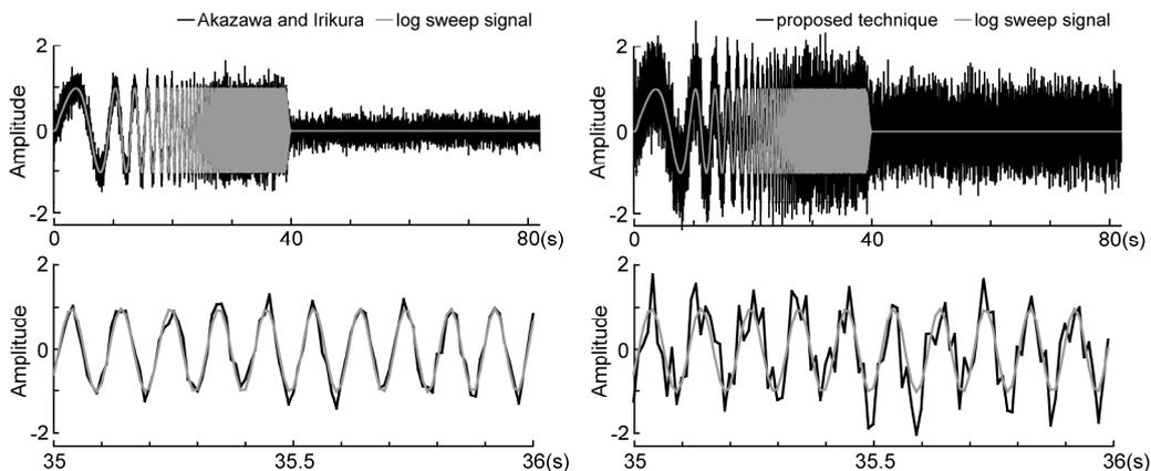
Fig.2 Waveforms obtained by Akazawa and Irikura (2007) procedure (left) and proposed technique (right).
