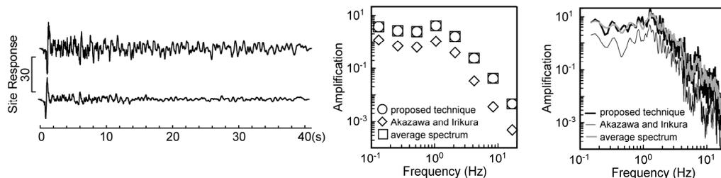
Fig.5 Obtained site amplification waveforms (left), site amplification wavelet spectra (center) and site amplification power spectra (right) for transverse component.
