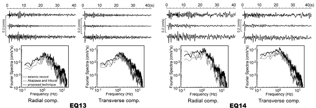
Fig.8 Velocity waveforms (top: seismic record, middle: (Akazawa and Irikura, 2007) procedure, bottom: proposed technique) and velocity Fourier spectra re-created for events unused in Section 5.2.
