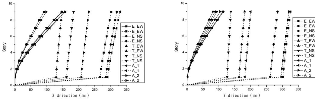
Figure 6 The max displacement of non-isolated structure and isolated structure
