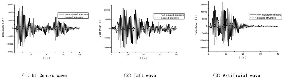
Figure 5 Time-history curve of base shear (Y Direction)
