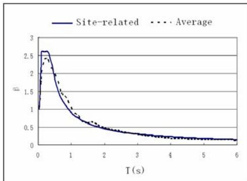
Figure 1 The curve of seismic effect coefficient (frequently- occurred earthquake)
