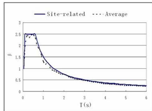
Figure 2 The curve of seismic effect coefficient (severe earthquake)
