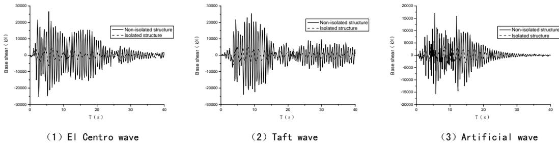
Figure 4 Time-history curve of base shear (X Direction)
