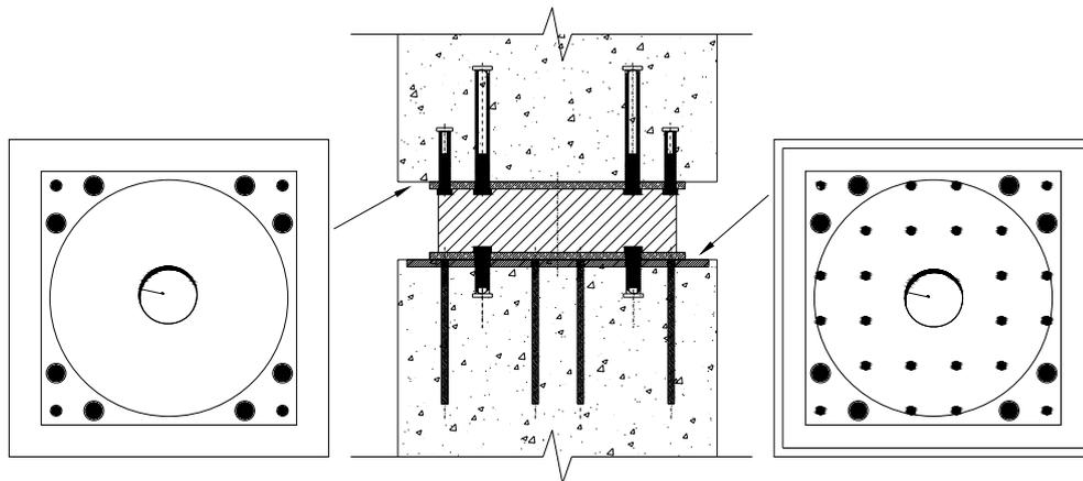
Figure 9 The connection between the rubber isolation bearing and structure
