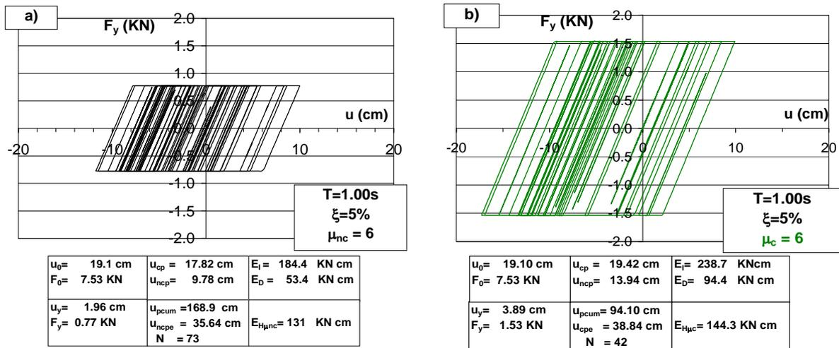
Figure 6. Hysteretic Responses for SDF's with  $T=1.00\text{s}$  subjected to the Llayllay Record of the Valparaiso 1985 Earthquake, for  $\mu_{nc} = 6$  (Fig. 6a) and  $\mu_c = 6$  (Fig. 6b)
