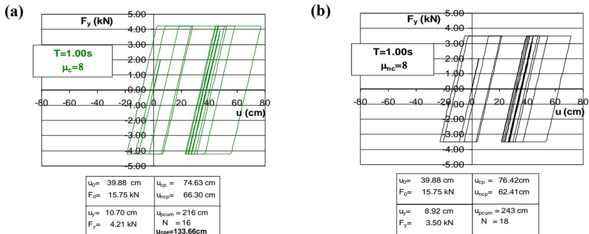
Figure 9. Hysteretic Response for SDFS with  $T=1.00$ s to the Takatori Record from Kobe 1995 Earthquake ; (a)  $\mu_c = 8$ ; and (b)  $\mu_{nc} = 8$
