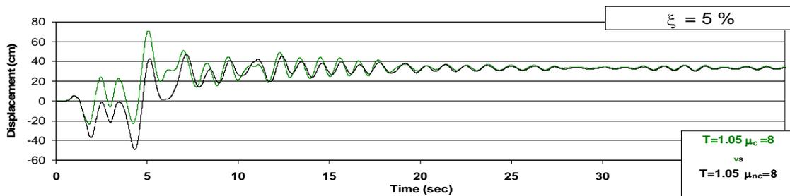
Figure 11b. Time History Response for SDFS with  $T=1.05s$  and  $\mu_c = \mu_{nc} = 8$  to the Takatori Record from Kobe 1995 Earthquake.
