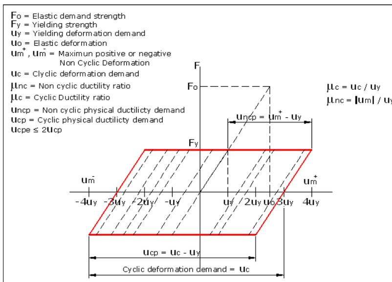
Figure 2. Elastic perfectly plastic force-deformation relationship.
