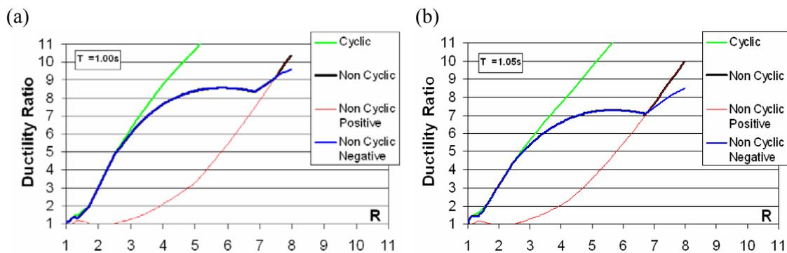
Figures 12a, 12b. Cyclic and non cyclic ductility ratio vs. strength reduction factors
