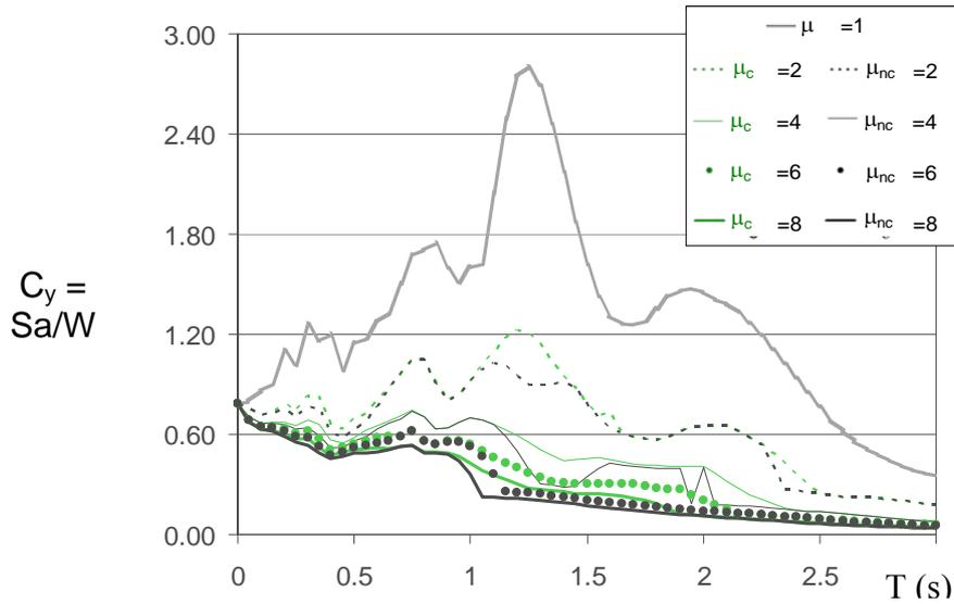
Figure 4. Cyclic and Non Cyclic Strength Demand Spectra for the 1995 Takatori record of the Kobe 95 earthquake.
