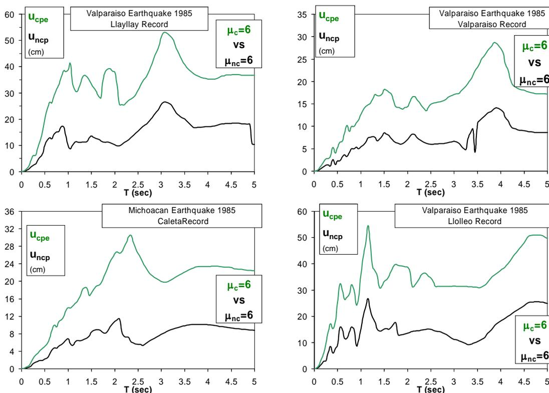
Figure 8. Cyclic Physical Ductility Demand Spectra and Non Cyclic Physical Ductility Demand Spectra for  $\mu_{nc}$  and  $\mu_c = 6$ .  $\xi = 5\%$ .
