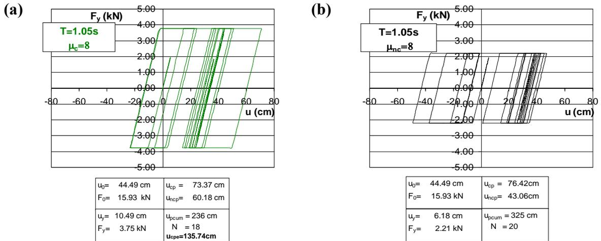
Figure 10. Hysteretic Response for SDFS with  $T=1.05s$  to The Takatori Record from Kobe 1995 Earthquake: (a)  $\mu_c = 8$ ; and (b)  $\mu_{nc} = 8$
