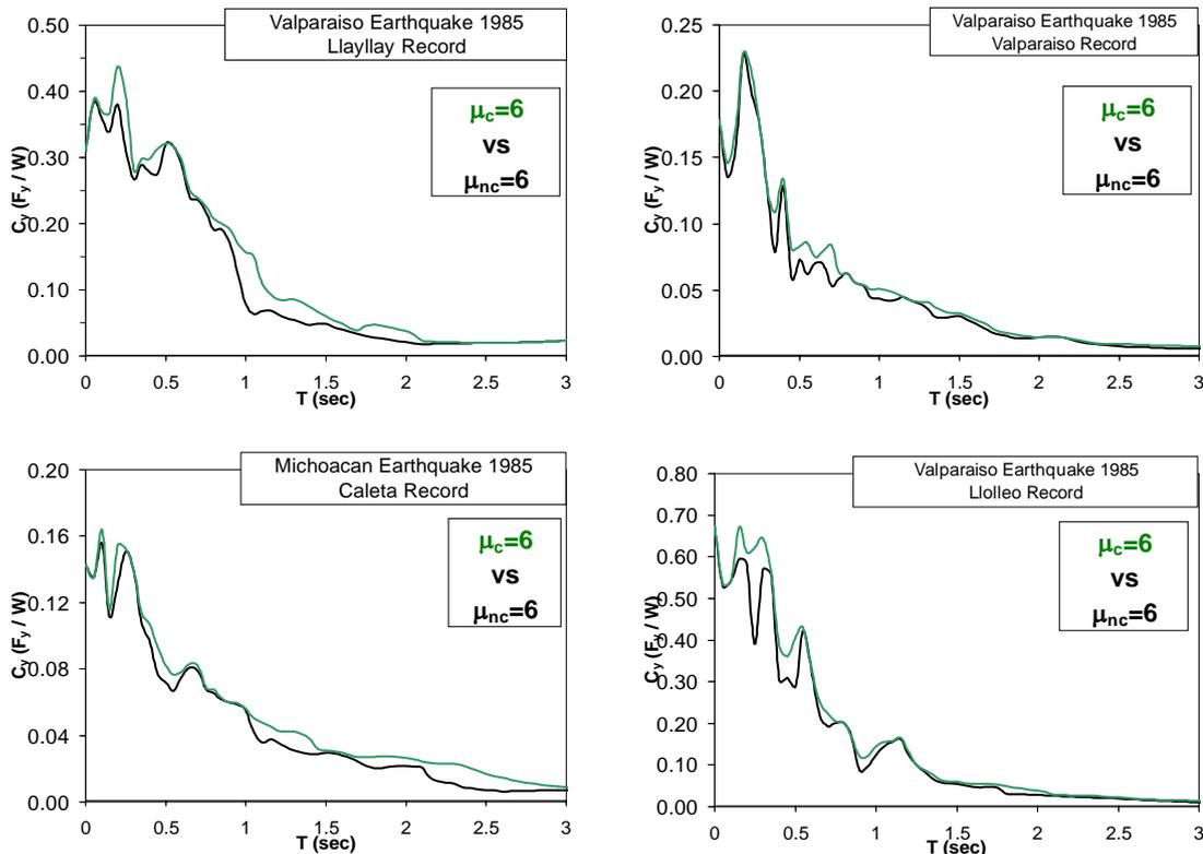
Figure 5. Cyclic and Non Cyclic Strength Demand Spectra for  $\mu_c$  and  $\mu_{nc} = 6$ .  $\xi = 5\%$
