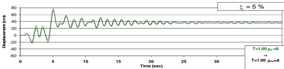
Figure 11a. Time History Response for SDFS with  $T=1.00s$  and  $\mu_c = \mu_{nc} = 8$  to the Takatori Record from Kobe 1995 Earthquake
