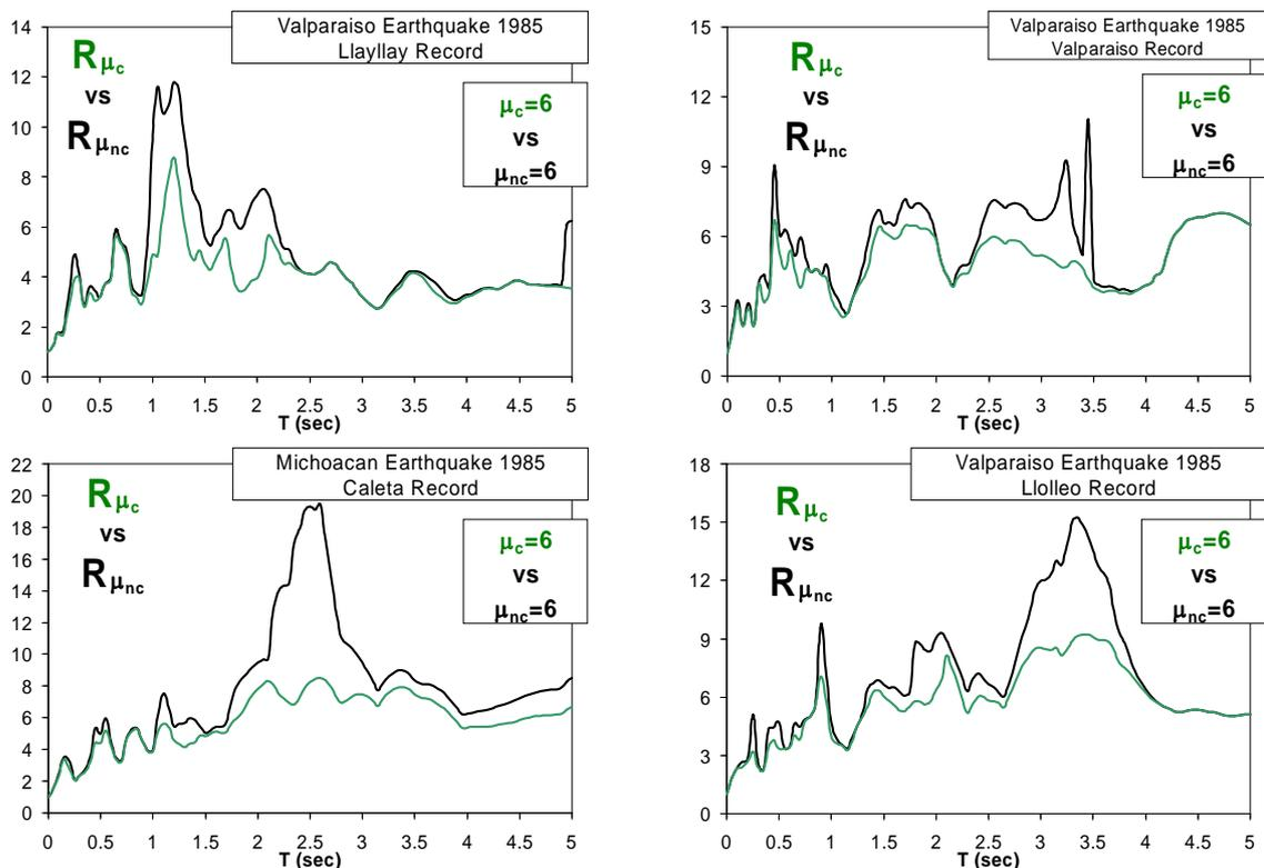
Figure 7. Cyclic and non cyclic strength reduction factor demand spectra for  $\mu_{nc} = \mu_c = 6$  and  $\xi = 5\%$
