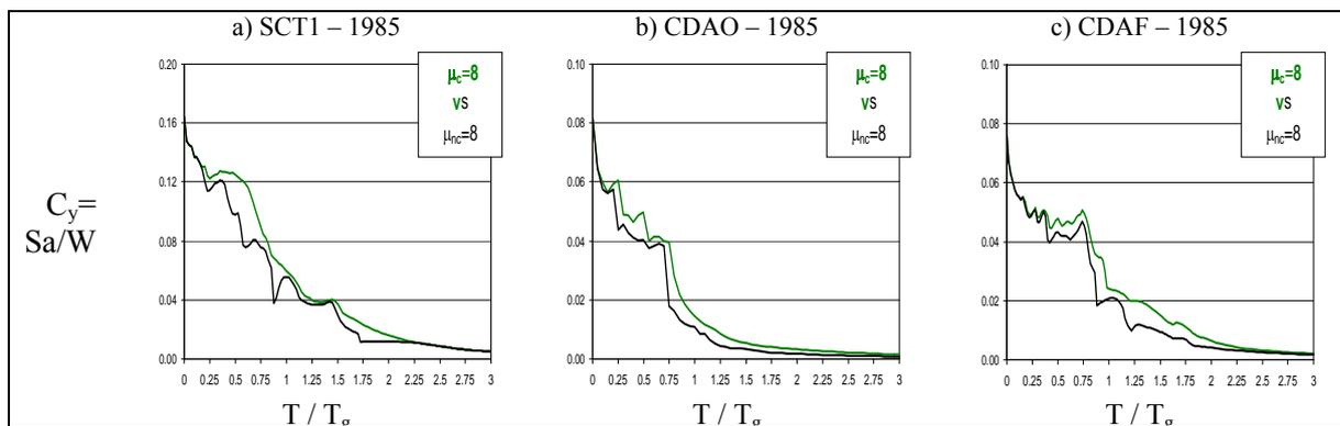
Figure 3. Cyclic and Non Cyclic Strength Demand Spectra for three records of the Michoacán, México 1985 earthquake ( $\xi = 5\%$ ).
