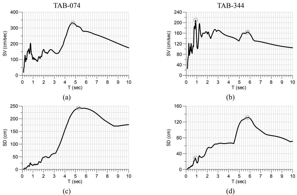
Figure 2. TAB-074 (left column) and TAB-344 (right column) components of Tabas, Iran, 1978 earthquake: (a) and (b) velocity spectra for  $\zeta=5\%$ ; (c) and (d) displacement spectra for  $\zeta=5\%$ .
