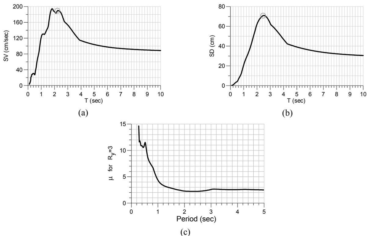
Figure 1. ERZ-000 component of Erzincan, Turkey, 1992 earthquake: (a) velocity spectrum for  $\zeta=5\%$ ; (b) displacement spectrum for  $\zeta=5\%$ ; (c) ductility demand spectrum for  $R_y=3$ .
