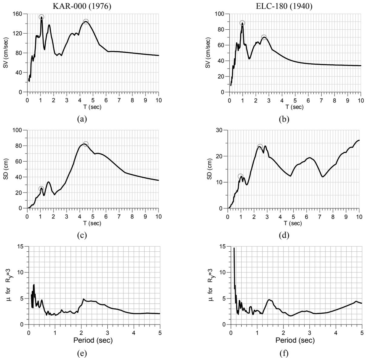
Figure 3. KAR-000 component of Gazli, USSR, 1976 earthquake (left column) and ELC-180 component of the Imperial Valley, USA, 1940 earthquake (right column): (a) and (b) velocity spectra for  $\zeta=5\%$ ; (c) and (d) displacement spectra for  $\zeta=5\%$ ; (e) and (f) ductility demand spectra for  $R_y=3$ .
