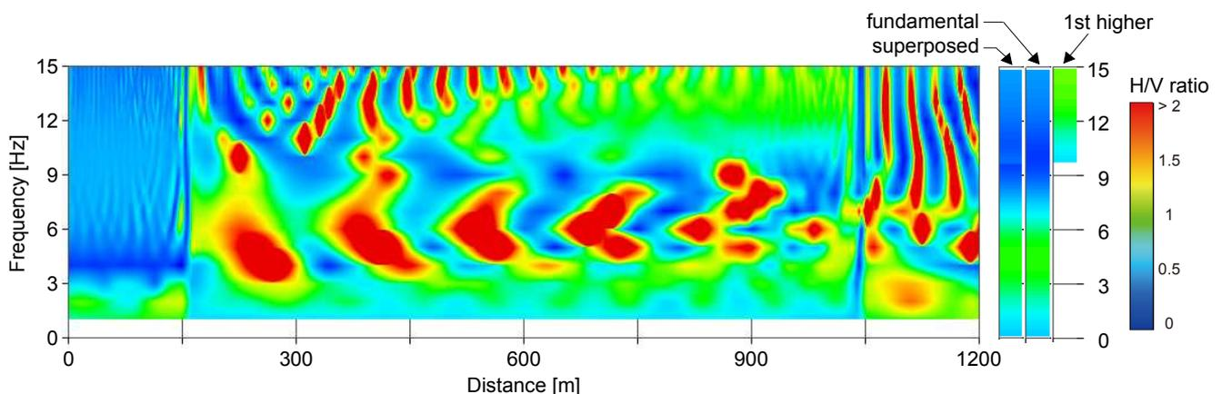
Figure 10 H/V spectrum along the ground surface (fundamental mode incidence)
