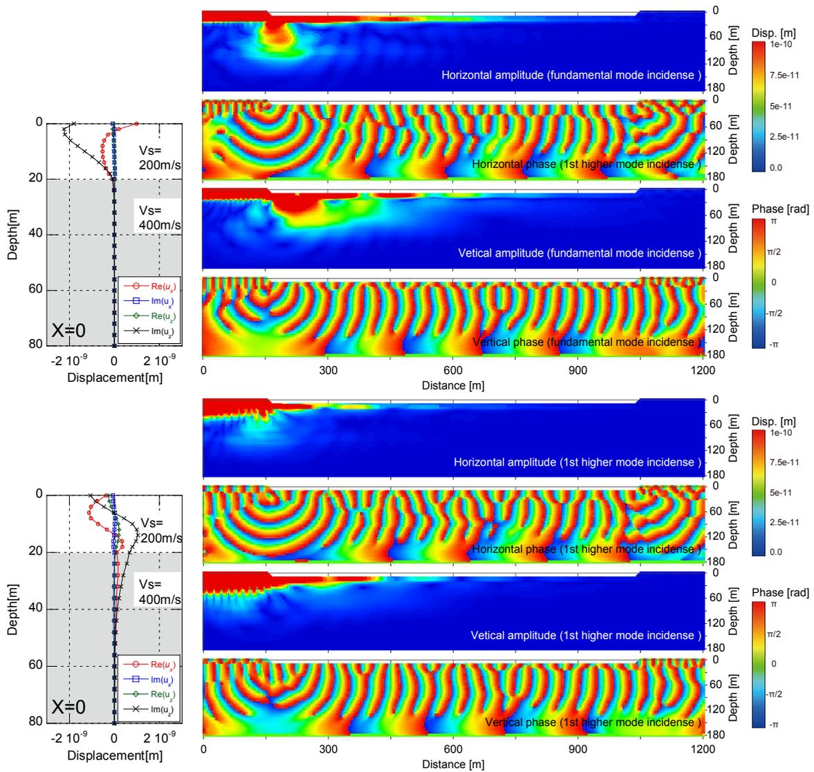
Figure 6 Rayleigh wave propagation in a valley shaped irregular ground for the frequency of 10Hz
