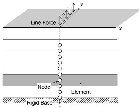
Figure 1 Thin layered element method
