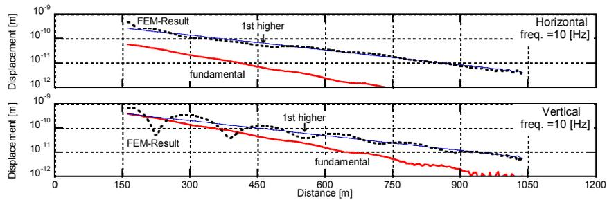
Figure 8 Contribution of the Rayleigh wave for the frequency of 10Hz (Fundamental mode incidence)
