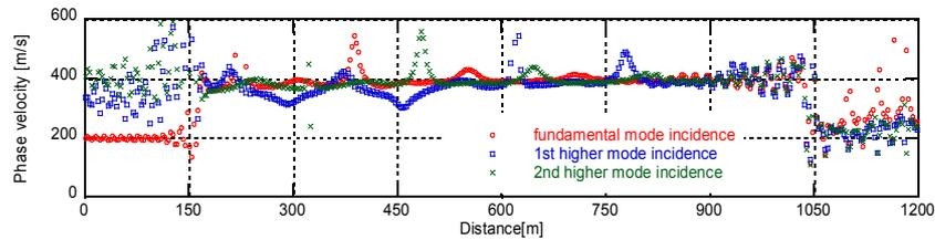
Figure 7 Phase velocity along the ground surface for the frequency of 10Hz
