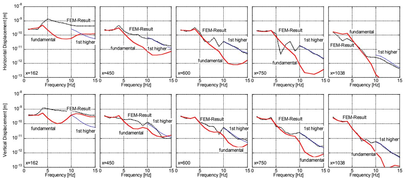
Figure 9 Contribution of the Rayleigh wave (fundamental mode incidence)
