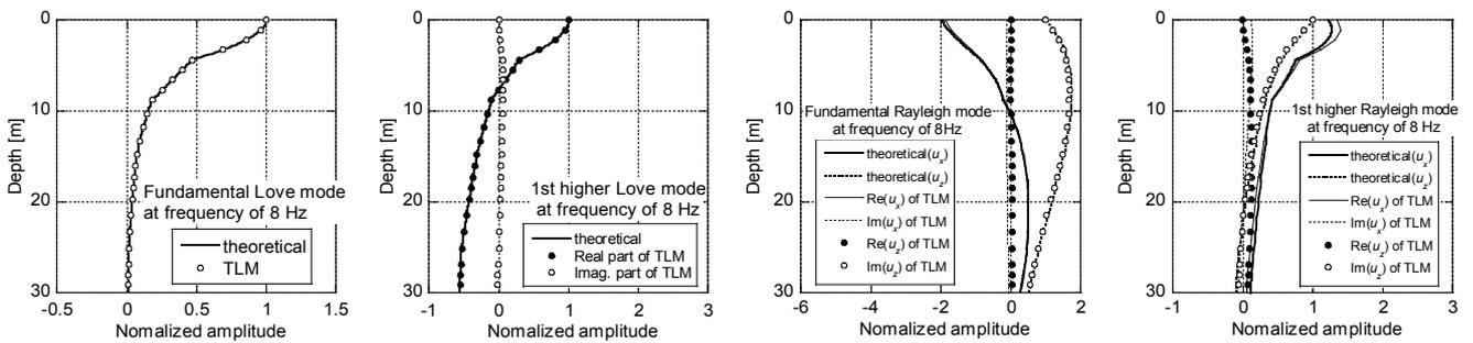
Figure 3 Comparison of mode shapes( $x=0$ ) for of 8Hz at site N
