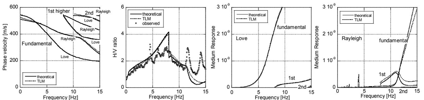
Figure 4 Comparison of phase velocities, medium responses, and H/V spectra at site N
