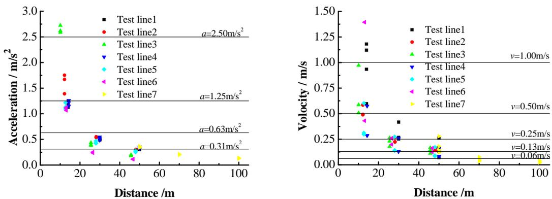
3 a. PGA and PGV of vertical direction with the distance to compaction point
