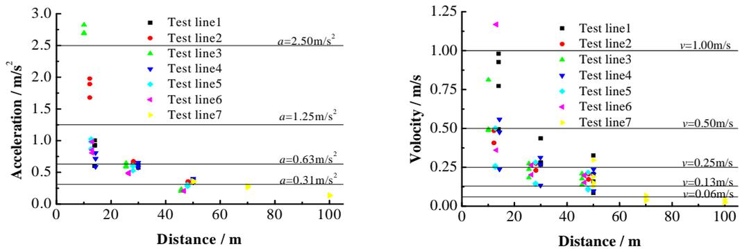
3c. PGA and PGV of north - south direction with the distance to compaction point
