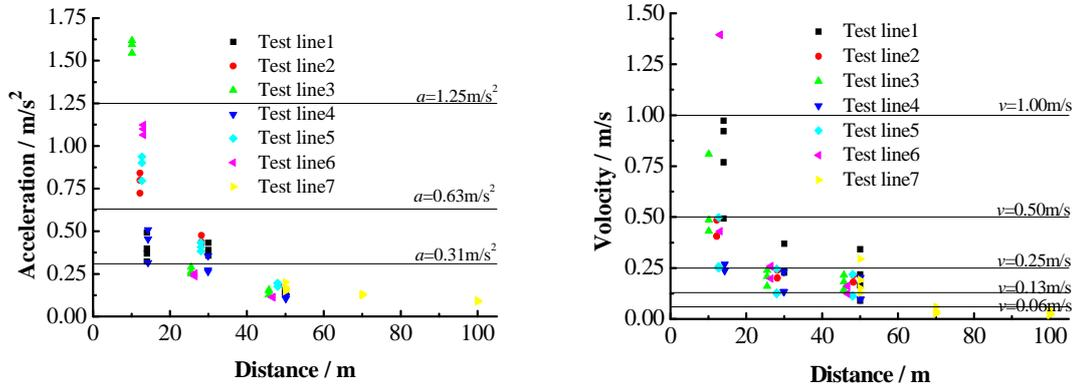
3b. PGA and PGV of east-west direction with the distance to compaction point
