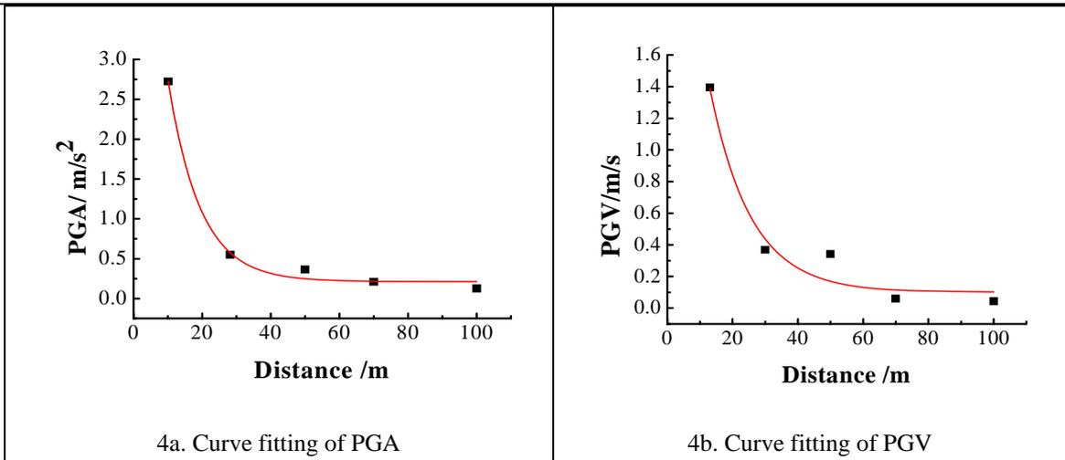
Figure 4 Curve fitting for peak values along vertical direction
