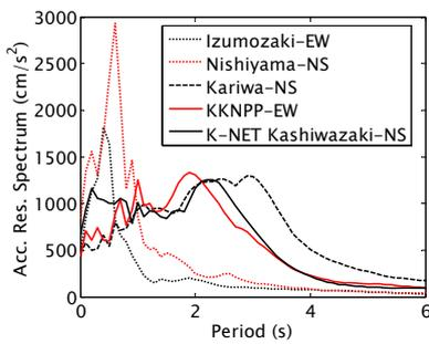
Figure 3 Response spectrum of acceleration.
