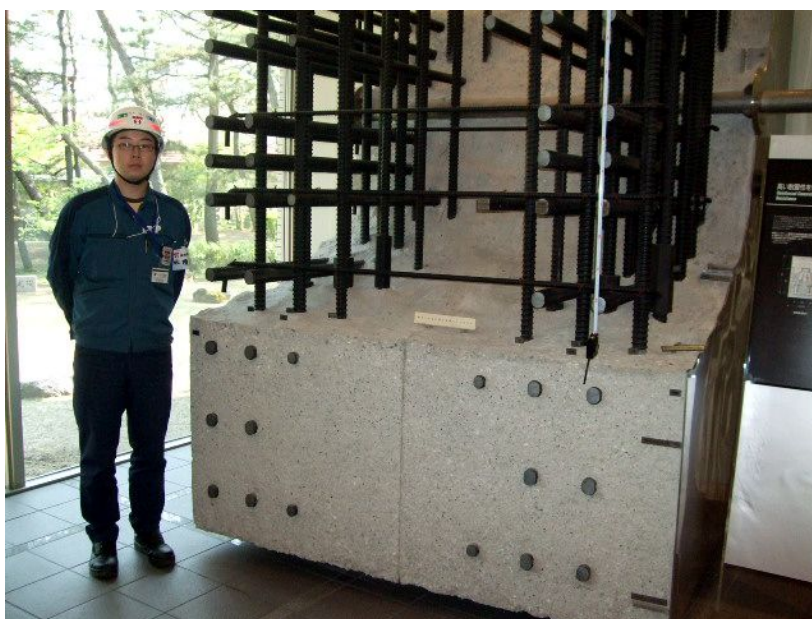
Figure 9 Reinforcing steel bars 51mm of diameter in the RC wall A lot of steel bars give the facilities a lot of “ductility”. by courtesy of TEPCO
