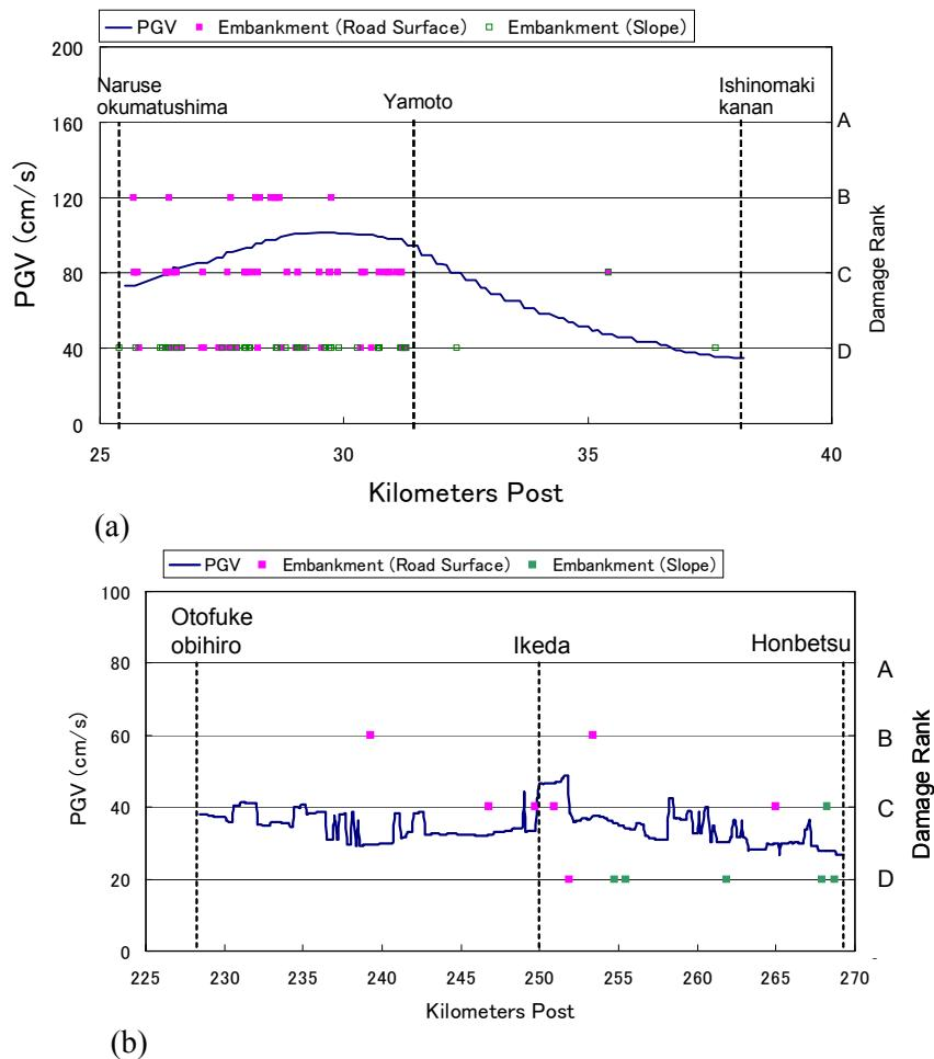
Figure 7 Relationship between the peak ground velocity and damages of expressway embankment for (a) the Sanriku expressway and (b) the Douto expressway embankment
