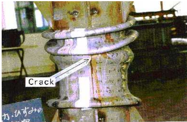
Figure 4: Deformation pattern of compression test
