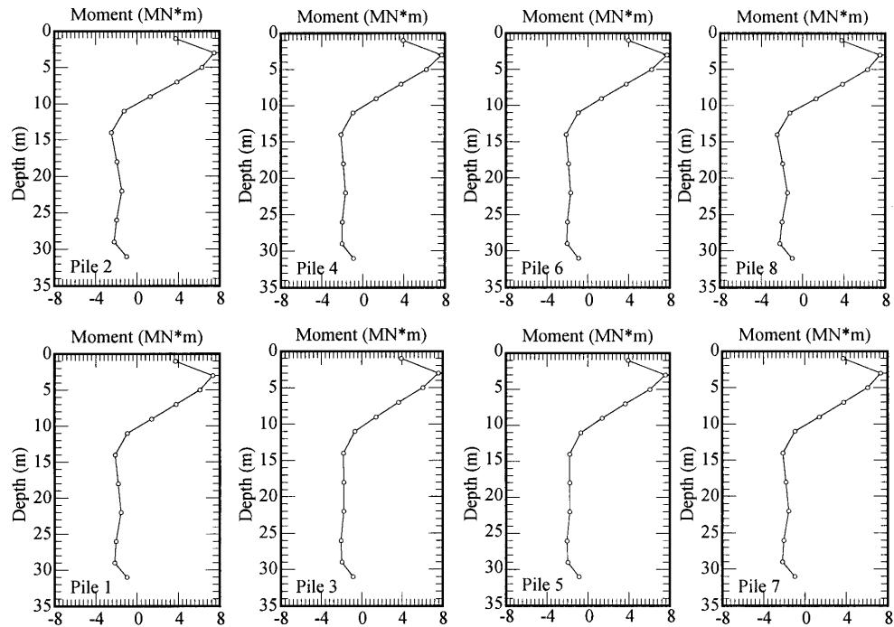
**Fig.9 Distribution of the moment in the piles (Elastic analysis,  $t=3.90$ )**
