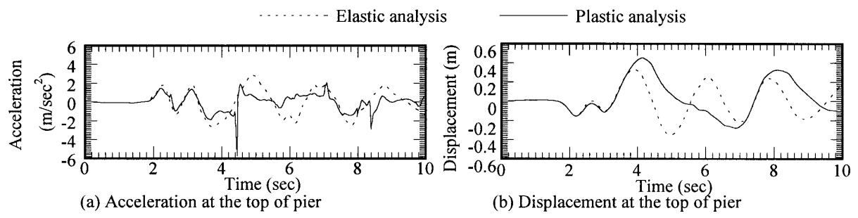
**Fig.8 Comparison of responding displacement and acceleration at the top of pier**
