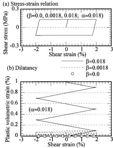
**Fig. 1 Stress-strain and stress-dilatancy relations in hollow cylindrical test with Drucker-Prager model**
