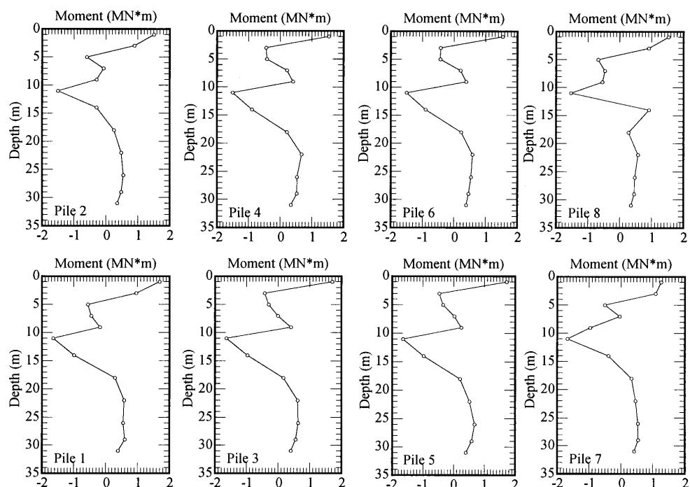
**Fig.10 Distribution of the moment in the piles (Plastic analysis,  $t=4.40$ )**
