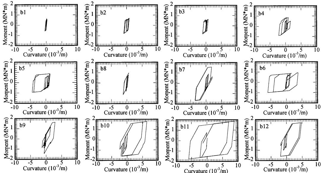
**Fig.13 Hysteresis of moment-curvature relation obtained from plastic analysis**
