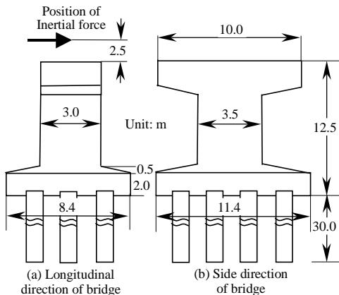
**Fig.4 Setup of group-pile foundation**
