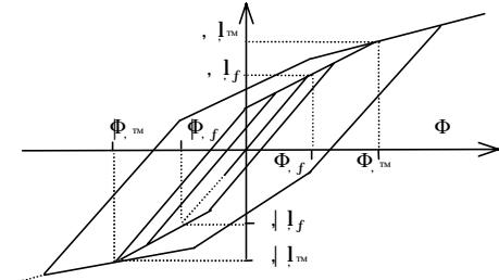
**Fig. 2 Tri-linear model for piles and pier**
