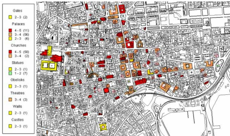
**Figure 6. Damage scenarios in Catania in terms of  $\mu_D$  (mean damage grade): 1693 earthquake.**
