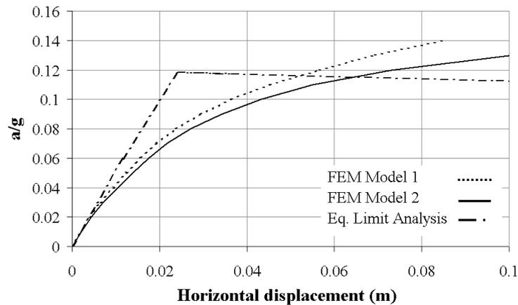
**Figure 11. Horizontal acceleration (in unit of g) vs. horizontal displacement - Model 1, 2 and ELA.**
