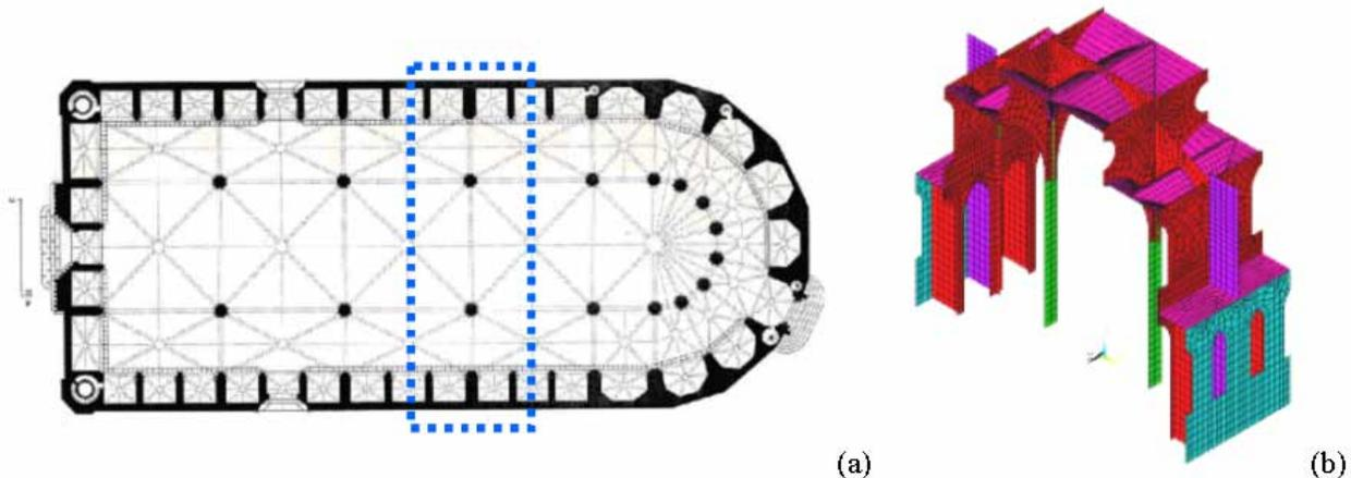
**Figure 10. (a) Plan view of the Church of S. Maria del Mar and the macroelement for the transversal response; (b) *FEM* model of the elements concurring to the transversal response.**
