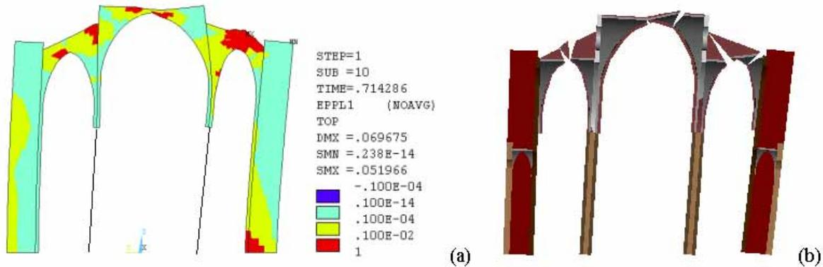
**Figure 12. (a) Inelastic maximum deformation; (b) Suggested kinematism.**
