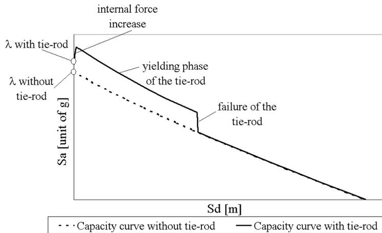
**Figure 8. Capacity curve behaviour with or without the tie-rod.**
