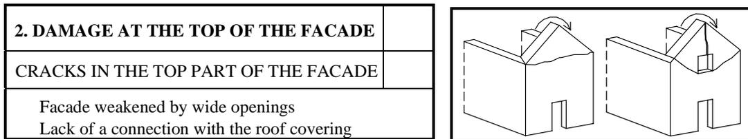
**Figure 1. An example of damage assessment in terms of macroelements and collapse mechanisms.**
