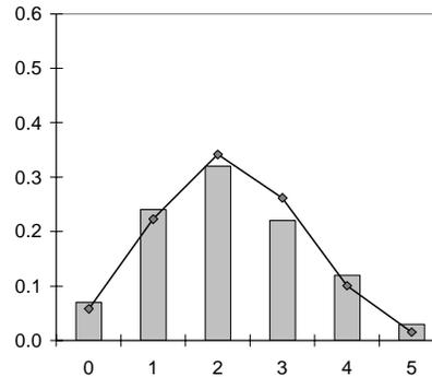
**Figure 4. Mean damage grade  $\mu_D$  and an example of damage grade distribution, function of a certain intensity (Umbria and The Marches earthquake, churches typology, intensity = VII).**
