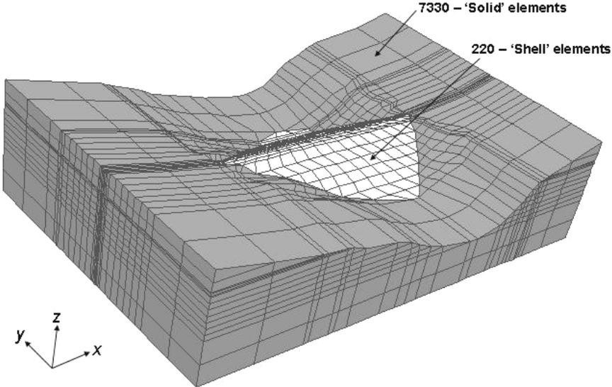
**Figure 3 Finite differences model 3-D of concrete face dam**
