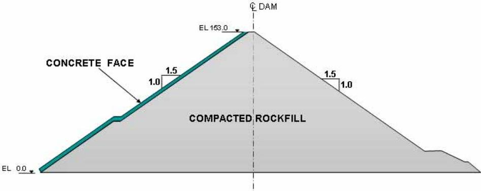
**Figure 2 Maximum section of concrete face rockfill dam**
