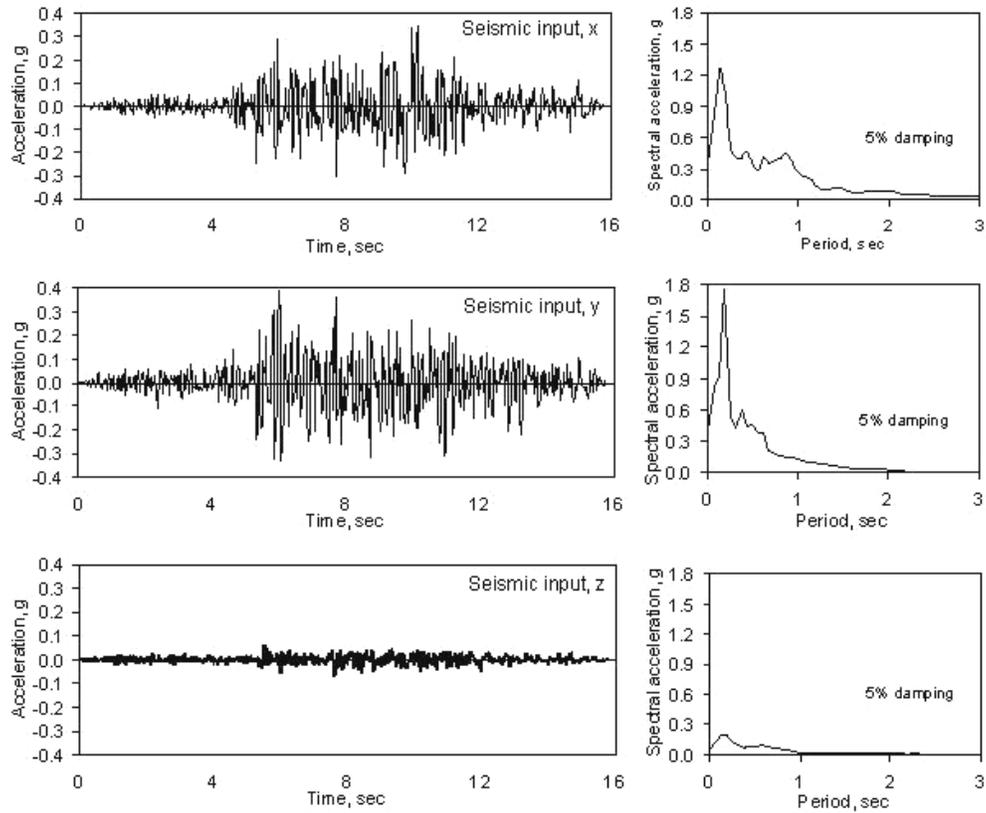
**Figure 4 Input recorded acceleration time histories and their response spectra**
