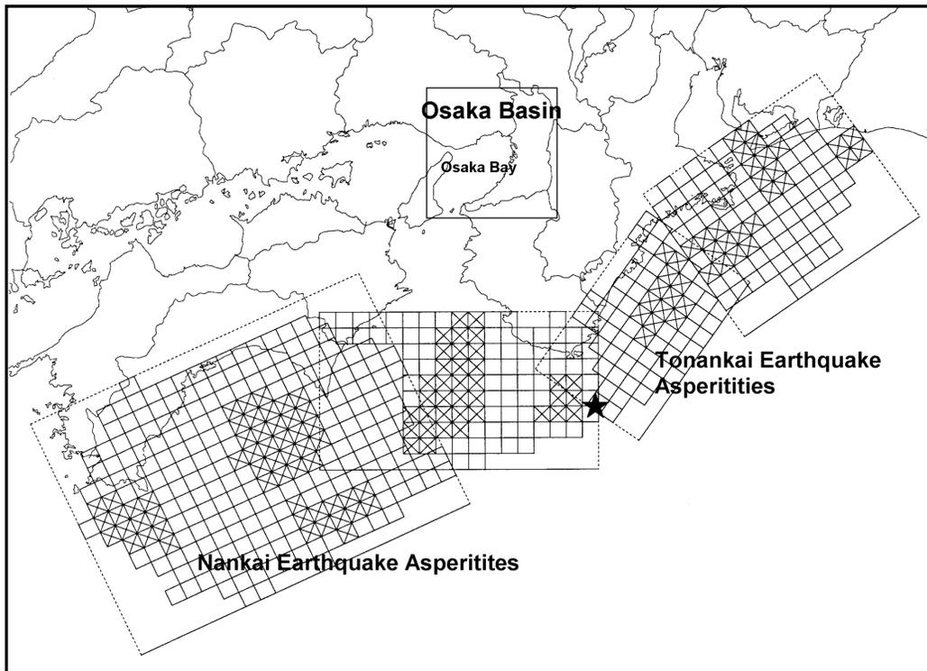
**Figure 5. Characterized asperity model for the Nankai and Tonankai earthquakes. Star indicates the rupture starting point used in this study.**
