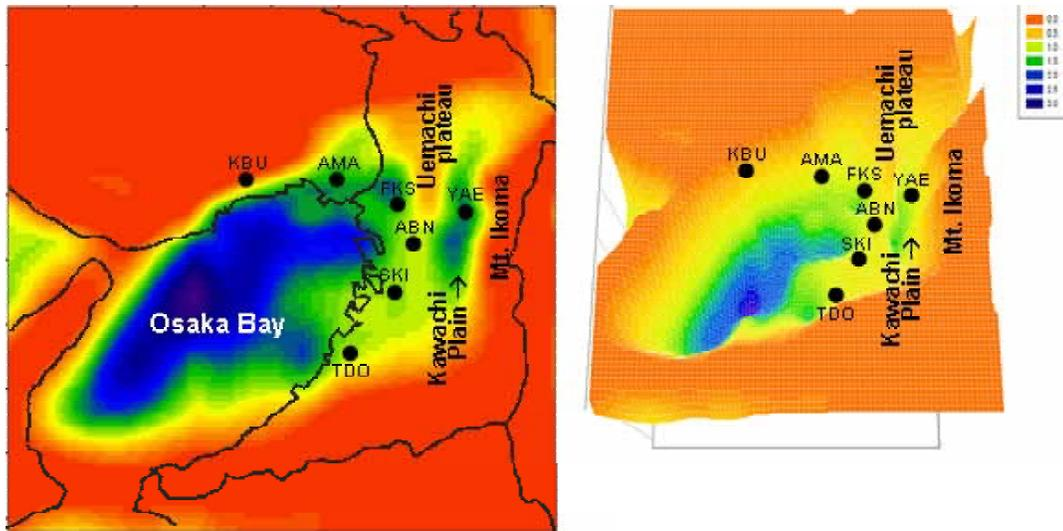
Figure 2. Three-dimensional Osaka basin structure (basement depth).
