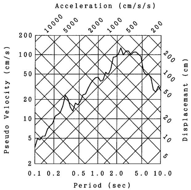
Figure 10a. The hybrid acceleration, velocity and displacement waveforms and their response spectrum (damping constant 5%) at ABN site.
