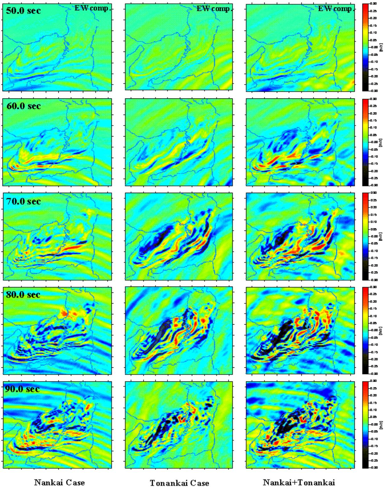
Figure 6. Snapshots of long period wave propagation through Osaka basin for the three cases. From left to right: case of occurrence of the Nankai earthquake, case of occurrence of the Tonankai earthquake and case of occurrence of the Nankai and Tonankai earthquakes simultaneously. Note difference of the wavelengths outside and inside basin.
