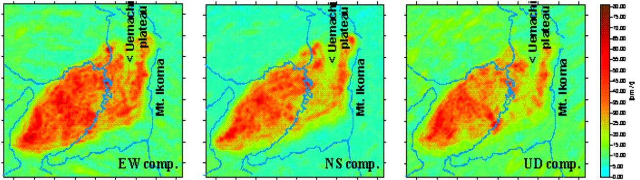
Figure 7. Peak ground velocity (*PGV*) distribution in Osaka basin for the three cases. From left to right: the Nankai earthquake, the Tonankai earthquake and the Nankai + Tonankai earthquake.
