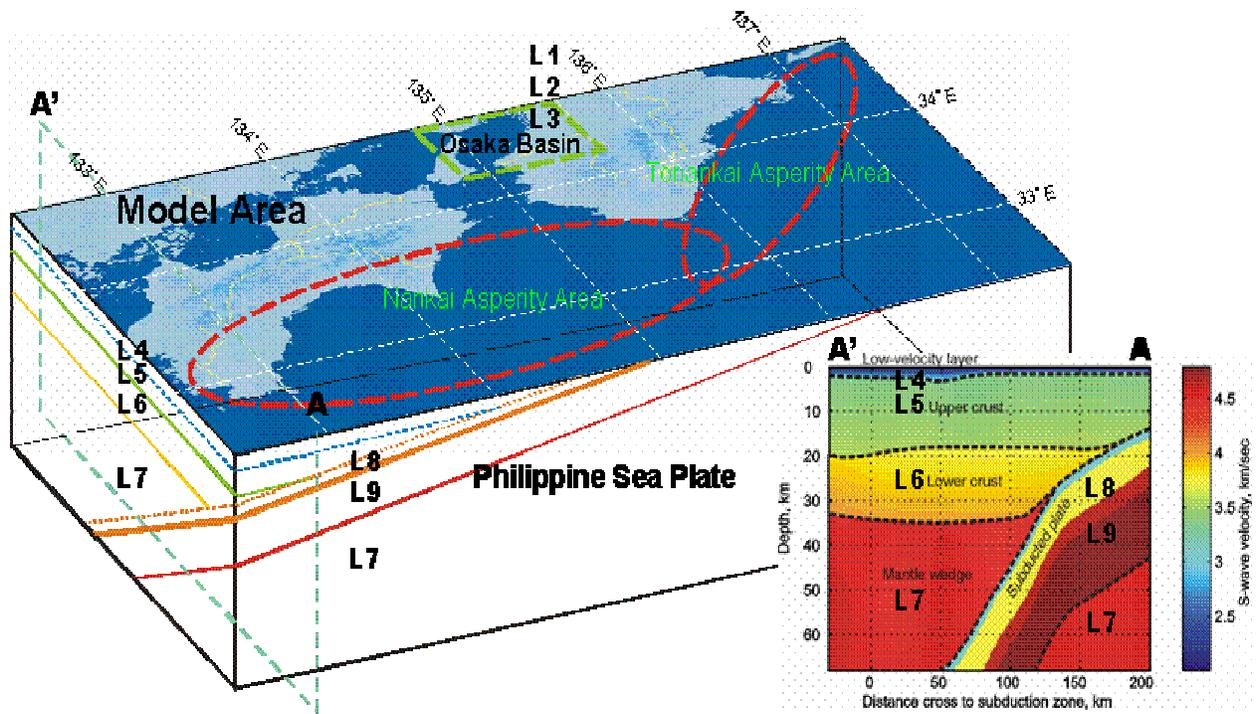
**Figure 1. Simulation area for the Nankai and Tonankai earthquakes. L1-L9 marks shows layered structure in Table 1.**
