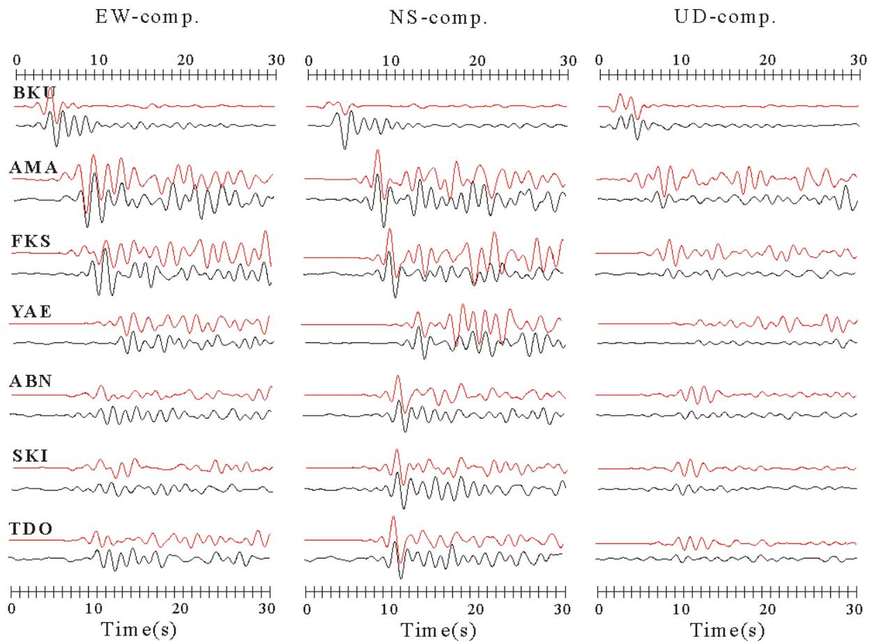
Figure 3. Comparison of three-component synthetic and observed velocity waveforms for a small earthquake. Red and black traces indicate synthesized and observed waveforms respectively. All waveforms are band-pass filtered in 0.1 - 1.0Hz.
