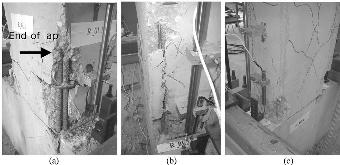
**Figure 8 Failure of R-type columns with lap-splices: (a) short - R-0L1, (b) medium - R-0L3, (c) long - R-0L4**
