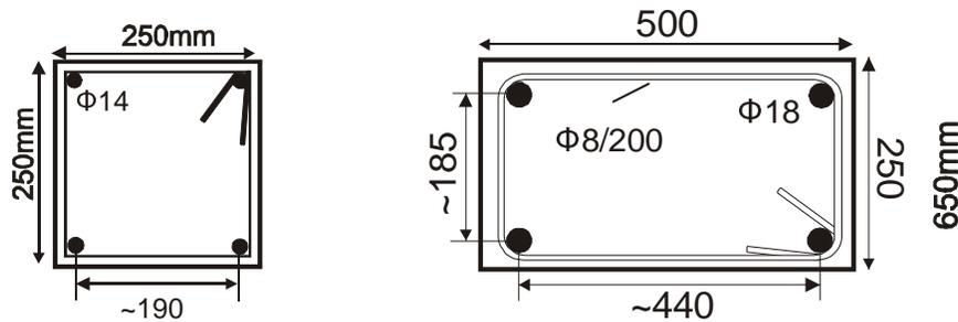
**Figure 1 Specimen cross-section and reinforcement**
