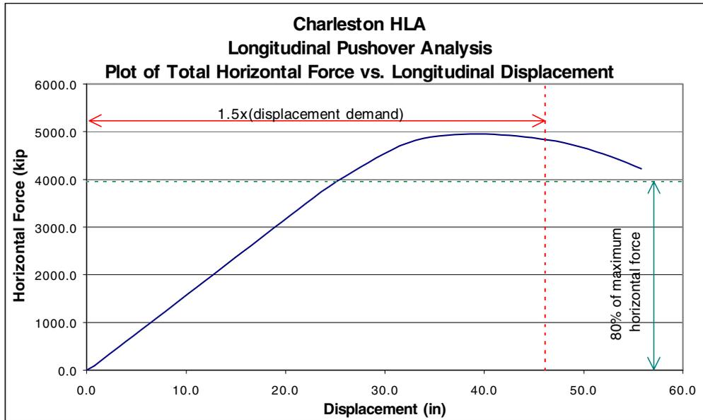
**Figure 8 – Force vs. Displacement Curve at Deck Level for Charleston High Level Approach**
