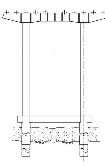
**Figure 4 – Typical Concrete Pier**
