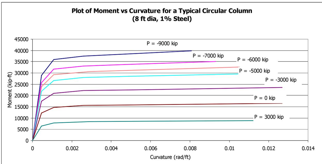
**Figure 7 – Moment-Curvature Curves for Column Section under Different Axial Force Levels**
