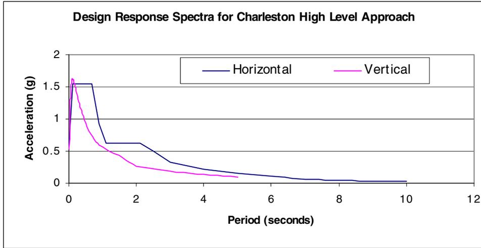
**Figure 1 – Design Response Spectra at Foundation for Charleston High Level Approach**
