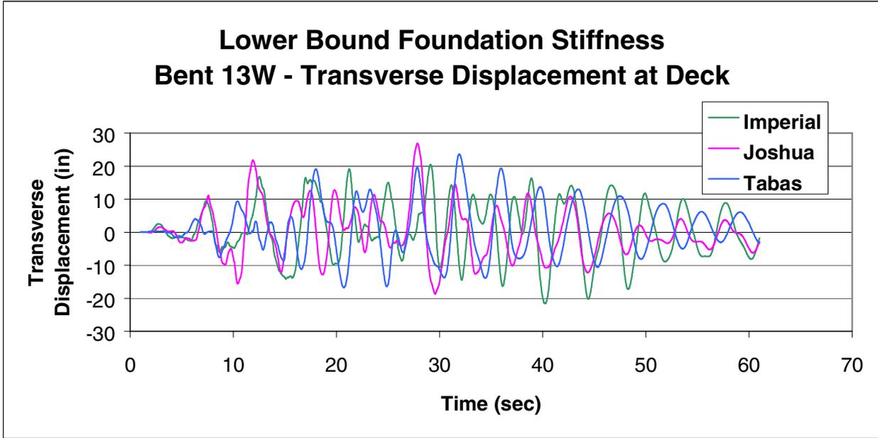
**Figure 11 – Transverse Displacement Response Time Histories at Deck Level for Pier 13W of Charleston High Level Approach**
