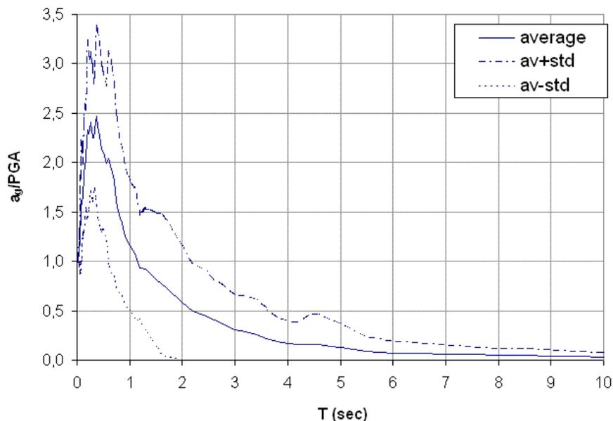
**Fig. 5: Response spectra (average, average +/- one standard deviation) for “bouquet A” of earthquake records (scalar Intensity Measure)**
