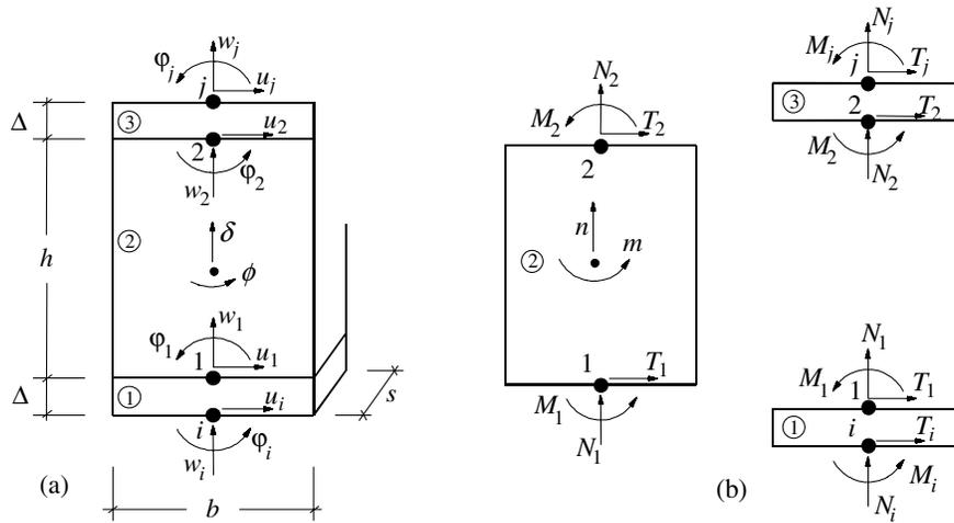
**Figure 4. Cinematic model for the macro element [6].**
