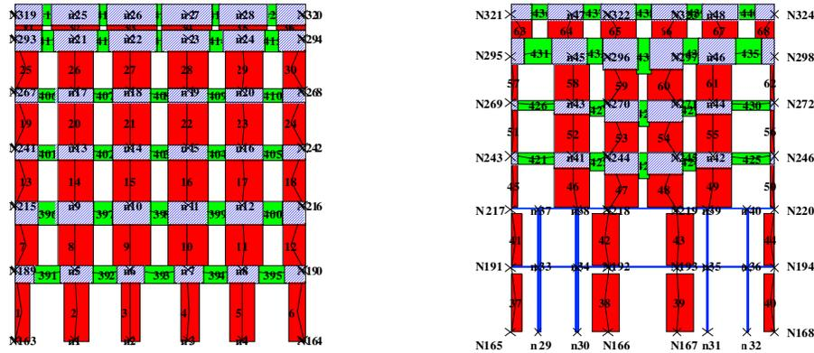
**Figure 7. Macro-element model. Walls 1 and 2.**
