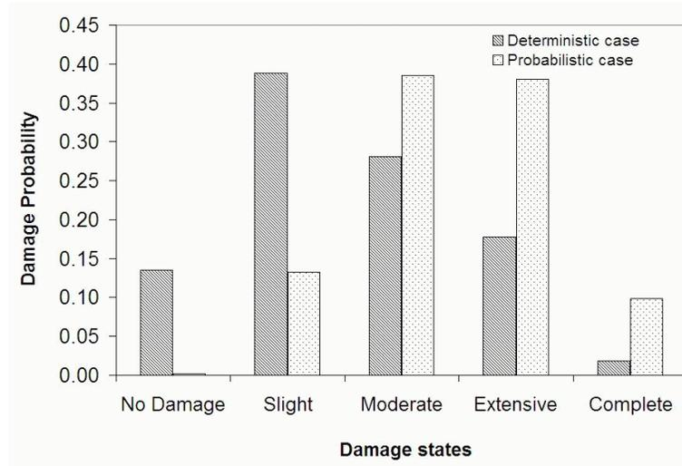
Figure 12. Damage probabilities for the deterministic and probabilistic seismic scenarios.
