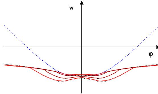
**Figure 5. Cyclic vertical displacement-rotation interaction with (red line) and w/o toe crushing (blue dots) [13]**
