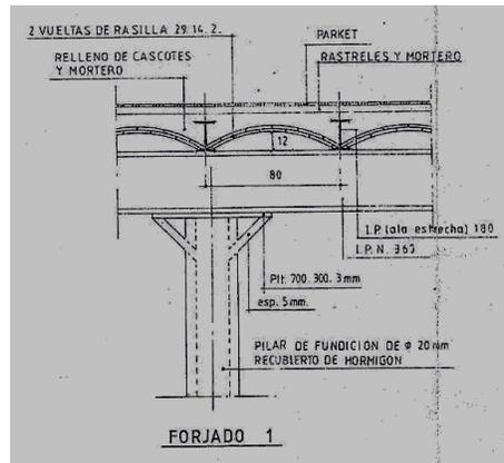
**Figure 1. Detail of the slab with steel beam and ceramics ceiling vaults (taken from the original architectonic plans of the building).**
