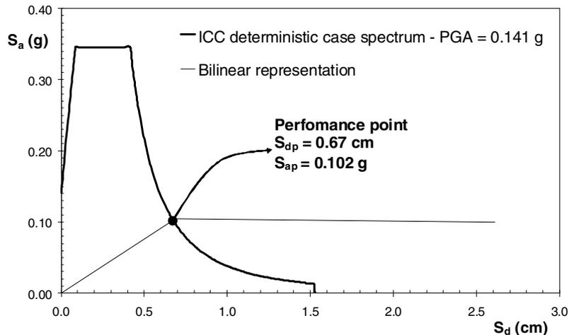
**Figure 9. Seismic performance point (deterministic case).**
