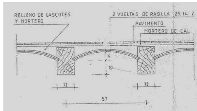
**Figure 2. Detail of the slab with wood beam and ceramics ceiling vaults (taken from the original architectonic plans of the building).**
