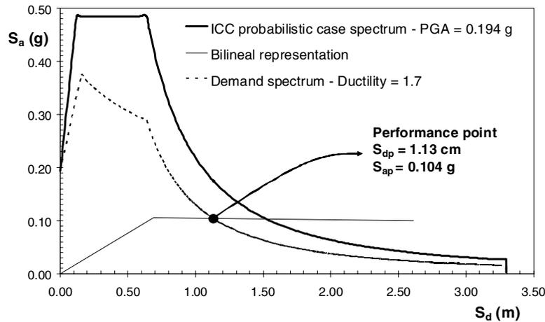
**Figure 10. Seismic performance point (probabilistic case).**
