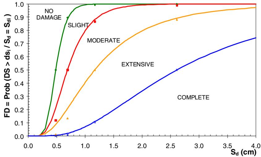
Figure 11. Fragility curves for six-story URM building of the Eixample .
