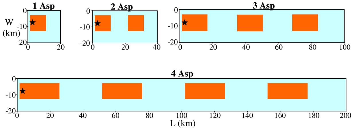
**Figure 4.** Rectangular asperity models for dynamic rupture simulation of surface earthquakes. Single asperity model is for  $L=W=20$ km, double for  $L=40$ km, triple for  $L=100$ km, and quadruple for  $L \geq 200$ km.  $L$  and  $W$  are the length and width of the fault, respectively. The star represents the hypocenter. The zero level is the free-surface.
