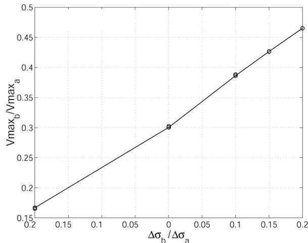
**Figure 3.** Relationship between the ratio of maximum slip-velocity ( $V_{max_b}/V_{max_a}$ ) with stress-drop ratio ( $\Delta\sigma_b/\Delta\sigma_a$ ) for the dynamic solution of a circular single asperity model with the asperity located at the center of the fault. The  $V_{max_a}$  and  $V_{max_b}$  are the average of maximum slip-velocity in the asperity area and in the back ground area, respectively.
