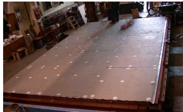
Figure 9: View of completed diaphragm test specimen with roofing.
