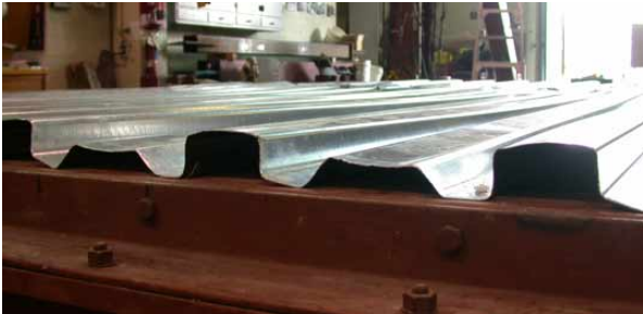
Figure 12: Warping deformations at the ends.
