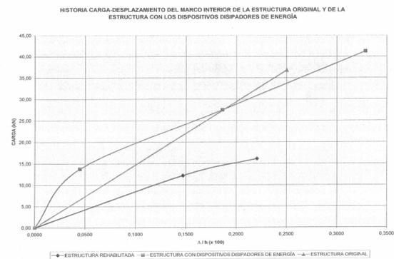
Figure 12 and 13 shows the lateral load displacement behavior structure-damper system of exterior and interior frames respectively. A stable hysteretic loops is observed for both frames also the stiffness and lateral capacity are sustained.
